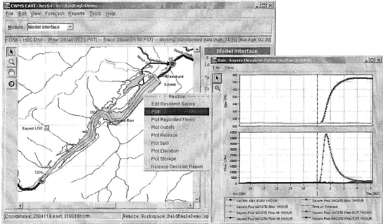
**Figure 6.** HEC-ResSim reservoir layer and sample display.
