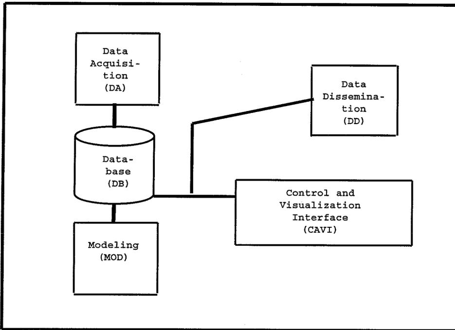
**Figure 1.** CWMS schematic and components.
