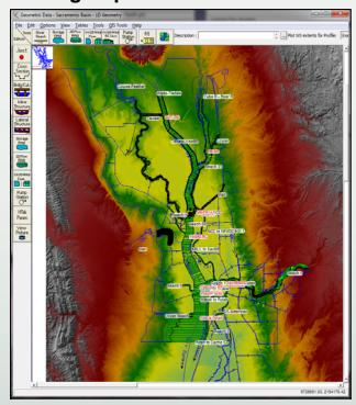
connections between two-dimensional flow & storage areas; pumping stations; floating ice; levees; extensive data import and export; and, geographic information system (GIS) connections.
