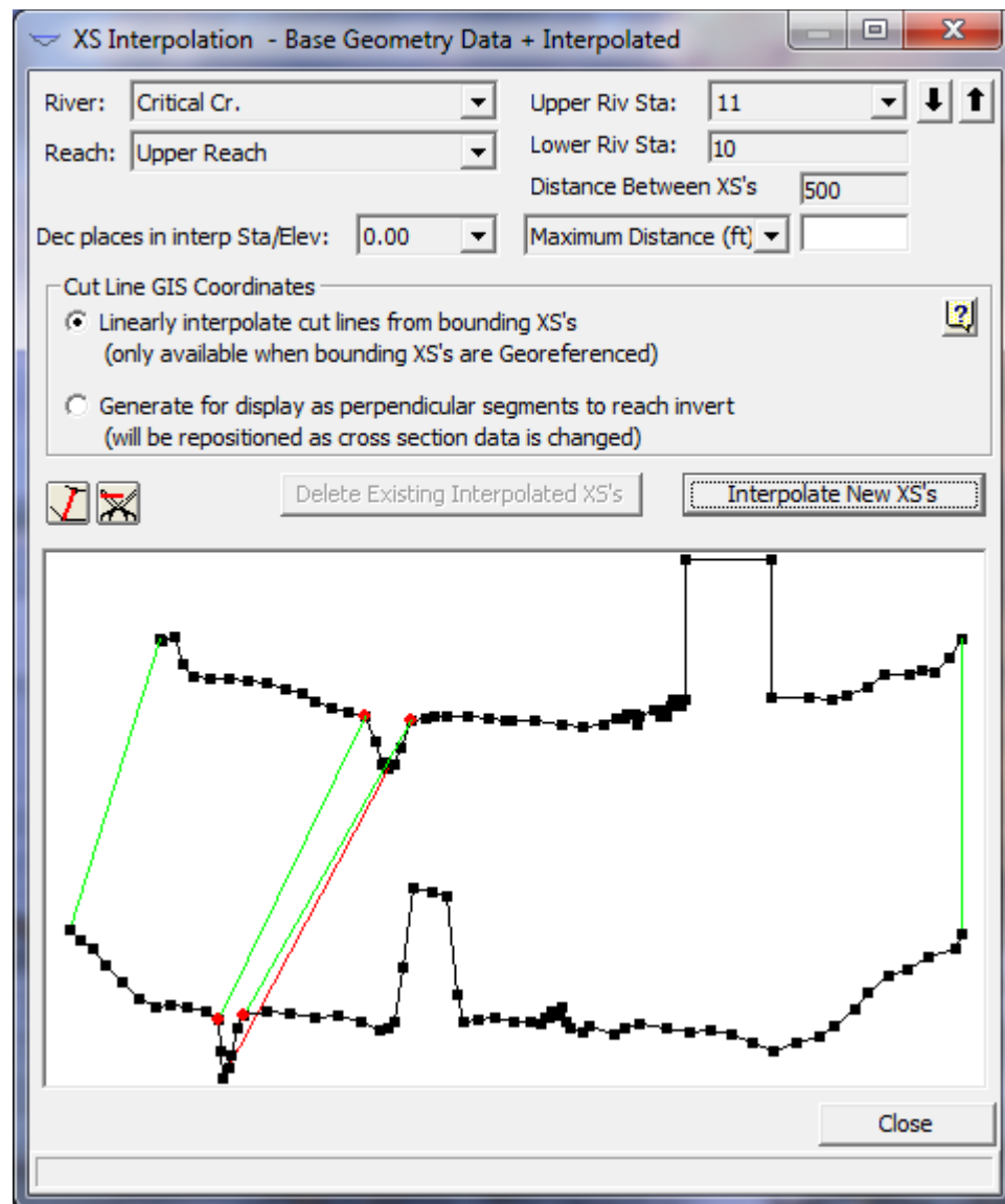
Figure 6-61 Detailed Cross Section Interpolation Window
