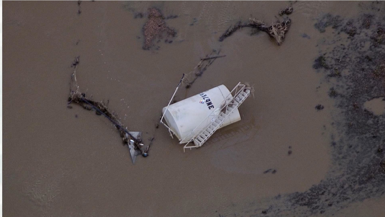
The 2013 Colorado Front Range Flood unseated and toppled several storage tanks, spilling thousands of gallons of crude oil. Weld County, CO 2013
