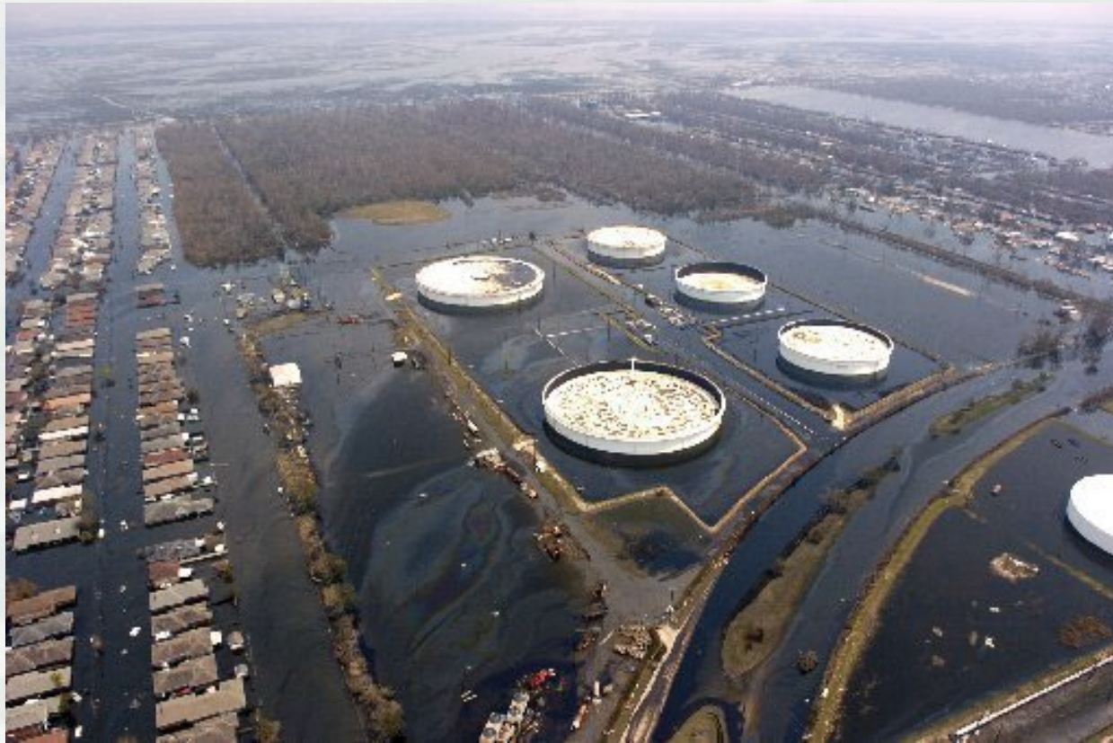
Storm surge from Hurricane Katrina moved a tank off its base at the Murphy Oil refinery, spilling over a million gallons of crude oil into floodwaters. St. Bernard Parish, LA 2005
