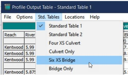
10. Compare the total overbank flow at the upstream cross-section (5.41) to the weir flow for the bridge.
