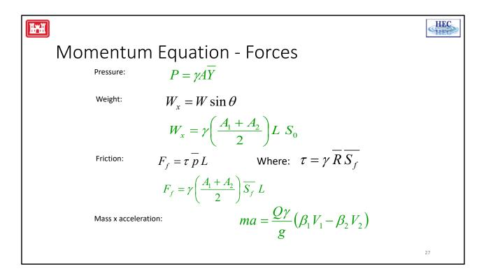
The assumption of a hydrostatic pressure distribution is only valid for slopes less than 1:10. The  $\cos\theta$  for a slope of 1:10 (approximately 6 degrees) is equal to 0.995. Because the slope of ordinary channels is far less than 1:10, the  $\cos\theta$  correction for depth can be set equal to 1.0 (Chow, 1959).
