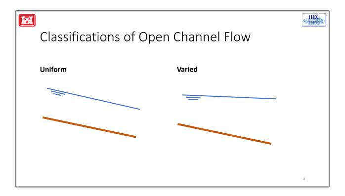
**Uniform Flow:** Depth and velocity are constant with distance along the channel.
