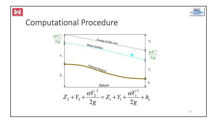
The following is the computational procedure for computing water surface profiles with the energy equation:
