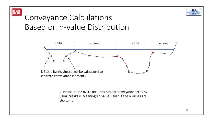
The two methods for computing conveyance will produce different answers whenever portions of the overbanks have ground sections with significant vertical slopes. In general, the HEC-RAS default approach will provide a lower total conveyance for the same water surface elevation.
