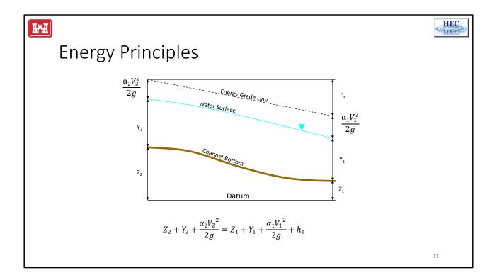
Water surface profiles are computed from one cross section to the next by solving the Energy equation with an iterative procedure called the standard step method. The Energy equation is written above.
