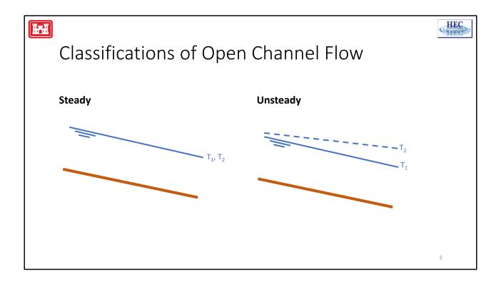
**Steady Flow:** Depth and velocity at a given location do not vary with time.
