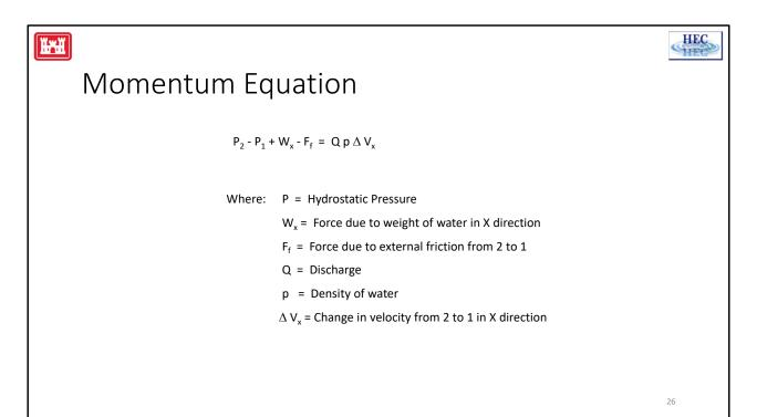
Applying Newton's second law of motion to a body of water enclosed by two cross sections at locations 1 and 2, the expression for the change in momentum over a unit time can be written as shown above.
