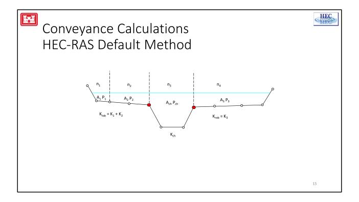
The default approach used in HEC-RAS for calculating conveyance is to subdivide flow in the overbank areas using the input cross section n-value break points (locations where n-values change) as the basis for subdivision. Conveyance is calculated within each subdivision from the Manning equation.
