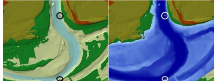
The elevation bumps circled above are likely due to data errors - and are really only visible if you zoom in. These errors, if unchecked, may affect the areas computed for different combinations of flow regimes and relationships. Especially when using different depth criteria.
