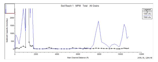
What is the range of transport capacities along the restored reach for the 2-yr flow? 0-20 tons/day
