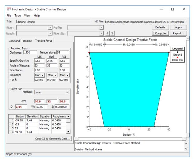
What are the minimum stable D75's for this channel: For a channel of D=7.44ft and W=50 ft
