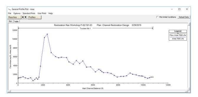
How do the velocity and area trends correspond to sediment capacity along the reach? **Sediment capacity is generally higher in areas of higher velocity and lower area.**
