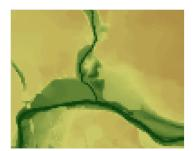
Terrain models are stored as either TINs or Grids. Triangulated Irregular Networks (TINs) are created by triangulating point data. TINs are the best way to represent a surface because they can represent linear features in the terrain using breaklines to enforce edges and elevations. In other words, you can densify information where elevations change rapidly (such as river banks or at levees). All ground surface models start as a TIN.
