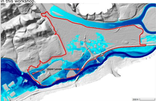
In this workshop, a 2D Connection will be added to the model and then a levee breach will be added.
