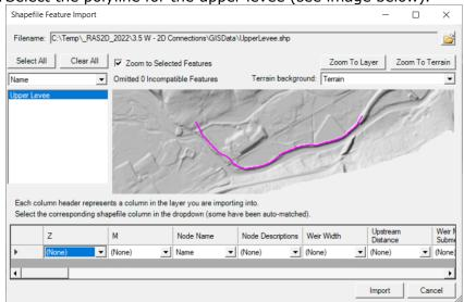
Note that Elevation data are not provided on the levee centerline.
