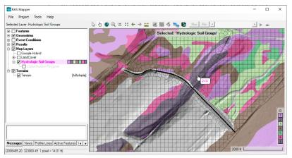
23. Create an Infiltration Layer by right-clicking on the Map Layer and selecting Create a New RAS Layer | Infiltration Layer From Land Cover / Soils Layers as shown in the figure below.
