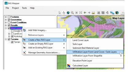
24. In the **Infiltration Layer** window, set the options as shown in the figure below and click **Create**. As mentioned previously, it is not necessary to utility both the Land Cover and Soils Layers for the SCS Curve Number method, but more accurate to do so.
