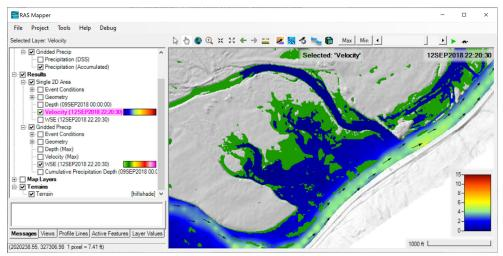
13. Add the **Cumulative Precipitation** result in **RAS Mapper** by right-clicking on the "Gridded Precip" plan and selecting **Create a New Results Map Layer...** from the menu.
