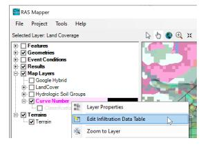
27. The **Classification Parameters** window will appear. The table contains all of the land classifications which need to be assigned SCS Curve Number infiltration parameters.
