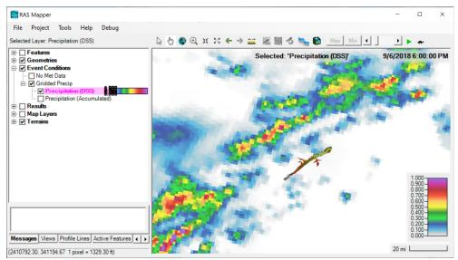
12. Inspect the HEC-RAS results and compare to the plans with and without precipitation. Use a different colormap for the water surface elevations highlight the differences or compare the extents of the water surface and velocity layers. See the example below.
