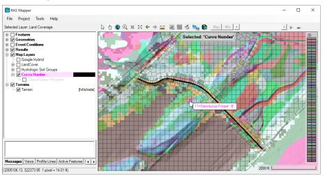
26. Right-click on the SCS Curve Number Infiltration Layer and select Edit Infiltration Data Table.
