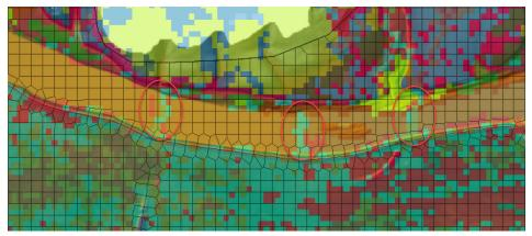
38. Practice fixing areas like this using **Classification Polygons**. Right-click on **Classification Polygons** and select **Edit Layer**. Then click on the **Add New Feature** tool **U**.
