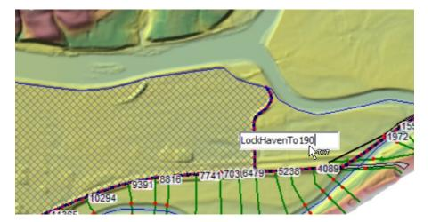
17. Using the **SA/2D Area Conn.** editor, connect the renamed connection to the the 2D Flow Area
