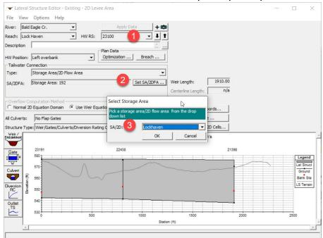
a. Notice that the plot displays the cell faces and the minimum cell elevation that the weir is connected to (you may have to switch the plot after hooking up the LS to LockHaven
