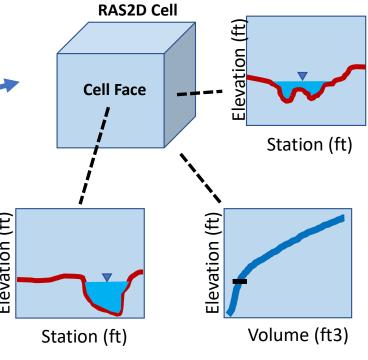
Each cell face profile and stage-volume curve is based on hundreds to thousands topo-bathymetric data-points, depending of resolution of underlying terrain raster.
