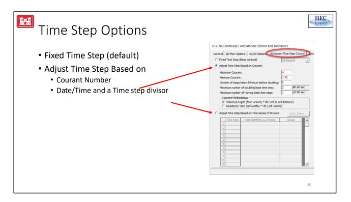
There are three options for the time step. The time step can be fixed for the entire run. The time step can be adjusted based on the courant number. The time step can be adjusted based on the date and time.
