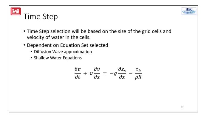
The 2D Computations in HEC-RAS support the Diffusion Wave approximation or Shallow Water Equations. The Diffusion Wave approximation is faster and more stable; however, is not a accurate a solution. In the DW approximation the friction slope is approximated by ignoring the local (due to time) and convective acceleration (due to change in location) (inertial) terms of the full SWE.
