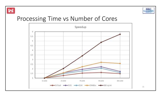
Shown are the results of testing a few data sets by running them with different numbers of Cores. Each model was run several times with the number of cores set to: 1, 2, 4, 8, and 16. As you can see four of the data sets had speed improvements up to 8 cores, but actually ran slower with 16 cores. These are smaller data sets ranging from 10,000 to 80,000 cells. However, one data sets had speed improvements all the way up to 16 cores. This was the largest data set, with 250,000 cells.
