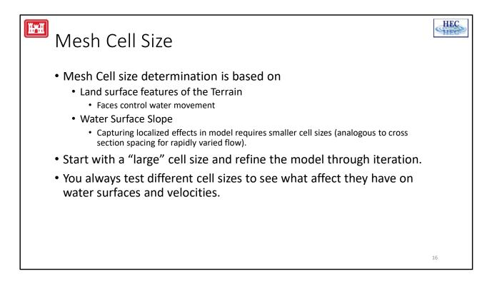
Cell faces should capture the detail in the terrain features that govern/direct the movement of flow. Because, RAS uses the cell faces as cross sections, cell size can vary though out the model, yet still produce accurate results despite having large cells.
