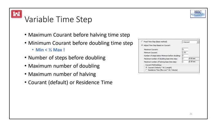
When using the courant option, for every time step RAS Unsteady will determine the maximum courant number by computing the courant number at every 1D cross section and at every 2D face.
