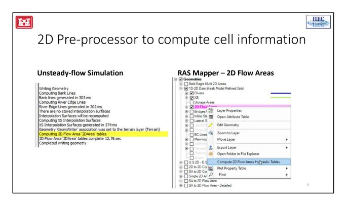
The 2D preprocess is accessed in RAS 2 different ways. The first way is that when a user runs a simulation, the 2D preprocessor is run to create hydraulic table information for each 2D Cell, if necessary. The second way is that users can access the preprocessor through RAS Mapper by right-clicking on the 2D Flow Area and selecting "Compute 2D Flow Area Hydraulic Tables".
