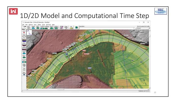
Here is an example where cross sections are spaced at 1000ft intervals (on average). It was determined that the 2D Grid Cell size should be 100ft (on average). To satisfy the Courant condition we consider spacing (cell size) and average velocities. If velocities are the same in the 2D Area as in the river, then we should choose a time slice that is 1000/100 or 10 (if we find velocities are typically much slower in the 2D Area, then we could use a smaller number of slices).
