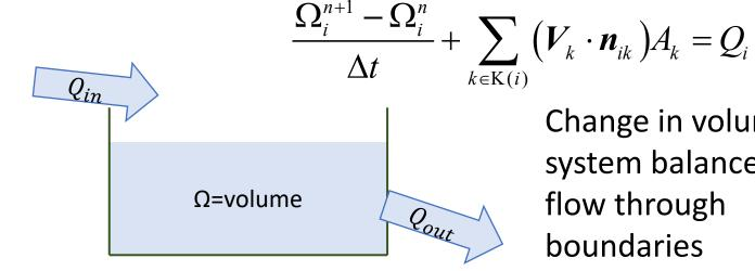
Change in volume in a system balances with flow through boundaries
