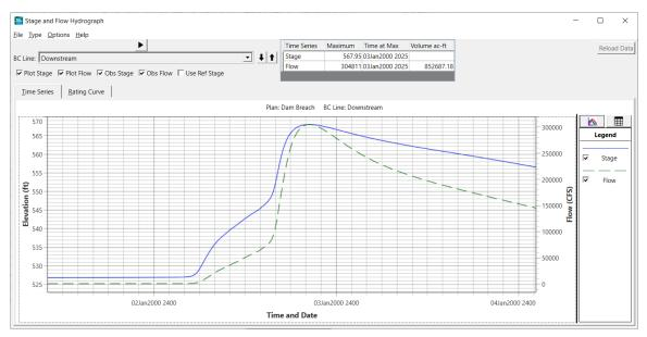
This flow is reasonable. Approximately, 200,000 cfs of peak flow was attenutated during the breach. The run time messages indicate a 0.026 percent volume error.
