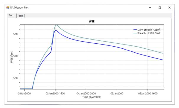
Another plot for the downsteam boundary. Peak stages are similar, however the DW solution has the floodwave arriving a bit sooner.
