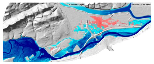
You can see the larger cell sizes allow water to spread faster.
