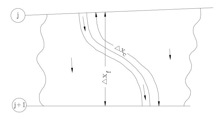
The reach length used for the floodplain area is computed by taking the arithmetic average of the left and right overbank reach lengths  $(L_L + L_R)/2 = L_F$ .
