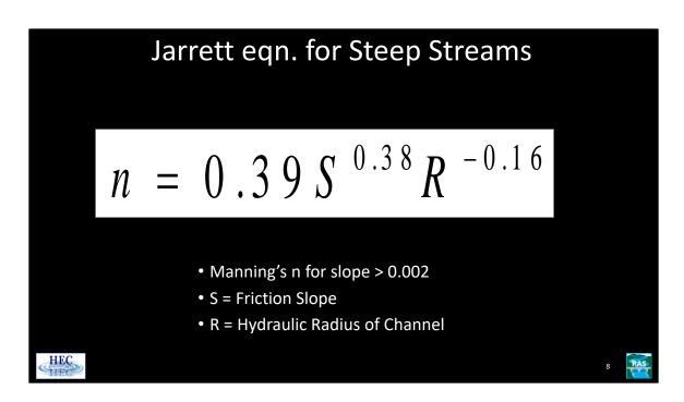
Because of the turbulence (that is otherwise not accounted for), Manning's n for steep streams is often higher than many user's realize. In addition to potentially more accurate results, the higher n value will generally improve stability. Jarrett (1984) developed an equation for high gradient streams (slopes greater than 0.002). Jarrett performed a regression analysis on 75 data sets that were surveyed from 21 different streams.
