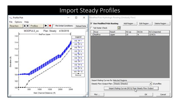
The MP method requires flow/water surface rating curve at every cross section in the MP region.
