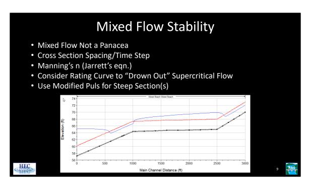
The mixed flow option does not guarantee that supercritical stretches will be stable. In areas that have rapidly changing depths and velocities, it is important to have close cross sections spacing. This includes the region upstream of critical depth (before the flow goes supercritical), the supercritical region itself, and the downstream hydraulic jump, if any.
