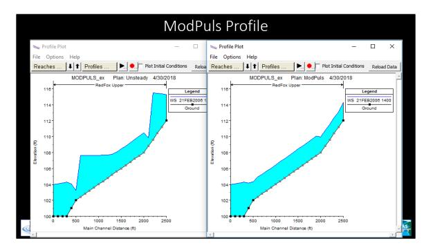
The profile on the left was performed using normal unsteady flow (and has gone unstable). The profile on the right is the same data with a MP region from the top (river station 25) to river station 4 (at 400 feet main channel distance).
