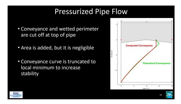
For most unsteady flow situations, water is treated as a non-compressible fluid. This is not strictly true. The volume of water in the slot can be thought of as the amount of water compressed under pressurized flow.
