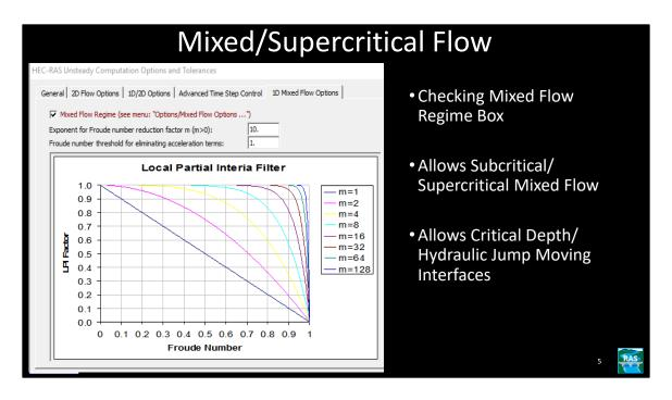
When the mixed flow option is checked, the program will modify the unsteady flow equations. This can increases model stability when there is subcritical flow, supercritical flow, hydraulic jumps, and/or draw downs (sub to supercritical transitions). This option should only be selected if you actually have a mixed flow regime situation.
