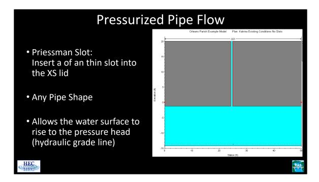
A Priessman slot can be added to any cross section that has a lid. From the Geometric editor, go to the Tables menu and select Priessman Slot.
