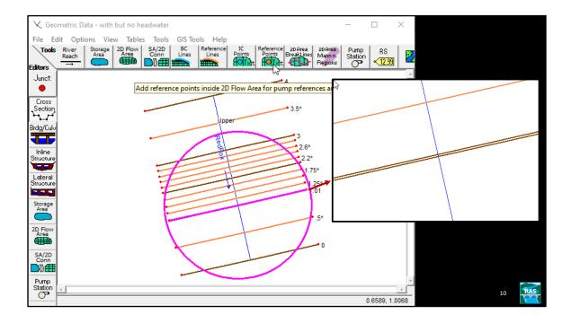
Care (and some experimentation) should be used in developing the rating curve. A higher rating curve will generally be more stable. However, a higher water surface could affect the results further upstream. For the profile on the right, the water surface almost touches critical depth. This should have minimal, if any, effect on the results further upstream. Steady flow experimentation may be quicker.
