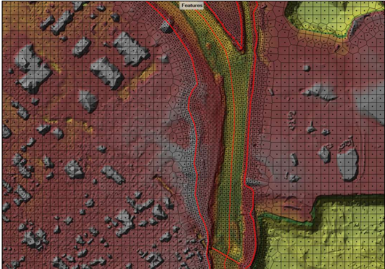
Figure 6-17. Example 2D mesh with a detailed mesh of the main channel, with grids aligned to the flow. Green to red color indicates the terrain (low to high elevation).
