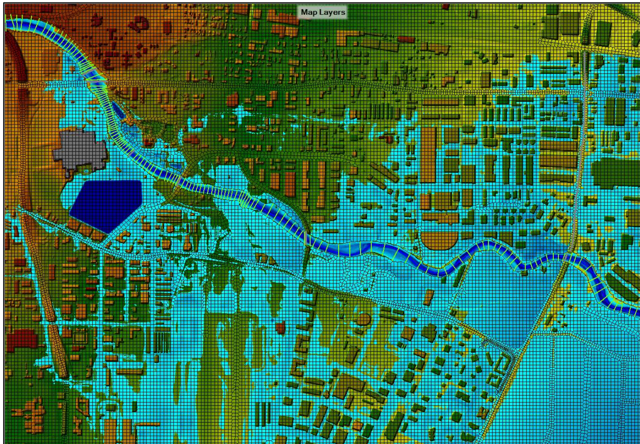
Figure 6-16. Example 1D/2D model of the Truckee River near Reno, NV. Green to red color indicates the terrain (low to high elevation) and the blues indicate water depth (dark blue indicates greater depth).
