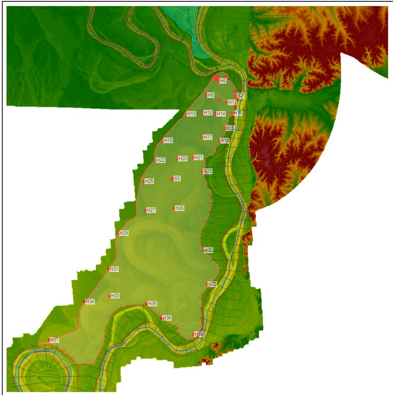
Figure 4-112. Combined One- and Two-Dimensional HEC-RAS Model of the Mississippi, Ohio, and New Madrid Floodway
