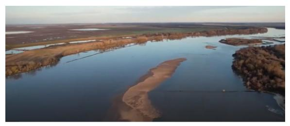
Then the District added four structures that increased the transport capacity, and this reach has not required dredging since. We will model a rising hydrograph with and without the structures and compute the difference in capacity to develop an understanding of how these structures affected capacity.
