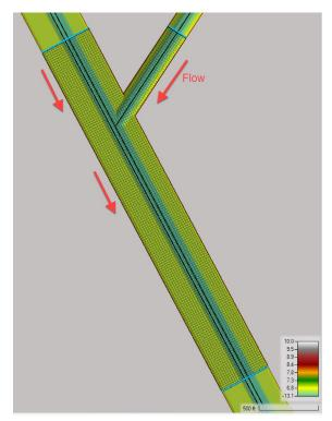
The model has flow boundary conditions upstream and a constant stage boundary condition downstream. The flow hydrographs vary for different plans depending on the specific processes being analyzed.
