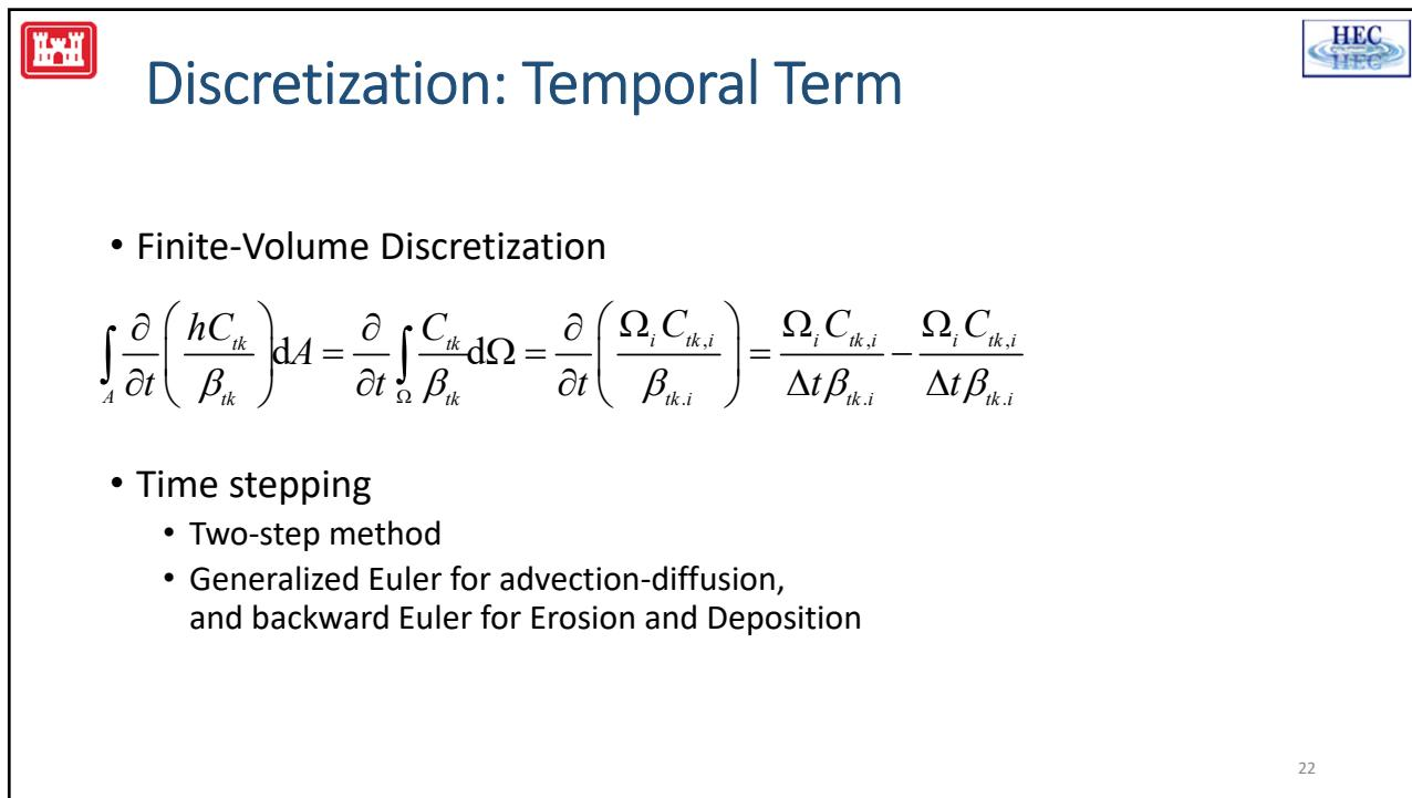
The screenshot shows the "Discretization: Temporal Term" dialog box from HEC-RAS. It details the finite-volume discretization of the temporal term, specifically the Crank-Nicolson scheme, which is a two-step method combining Generalized Euler for advection-diffusion and backward Euler for Erosion and Deposition.
