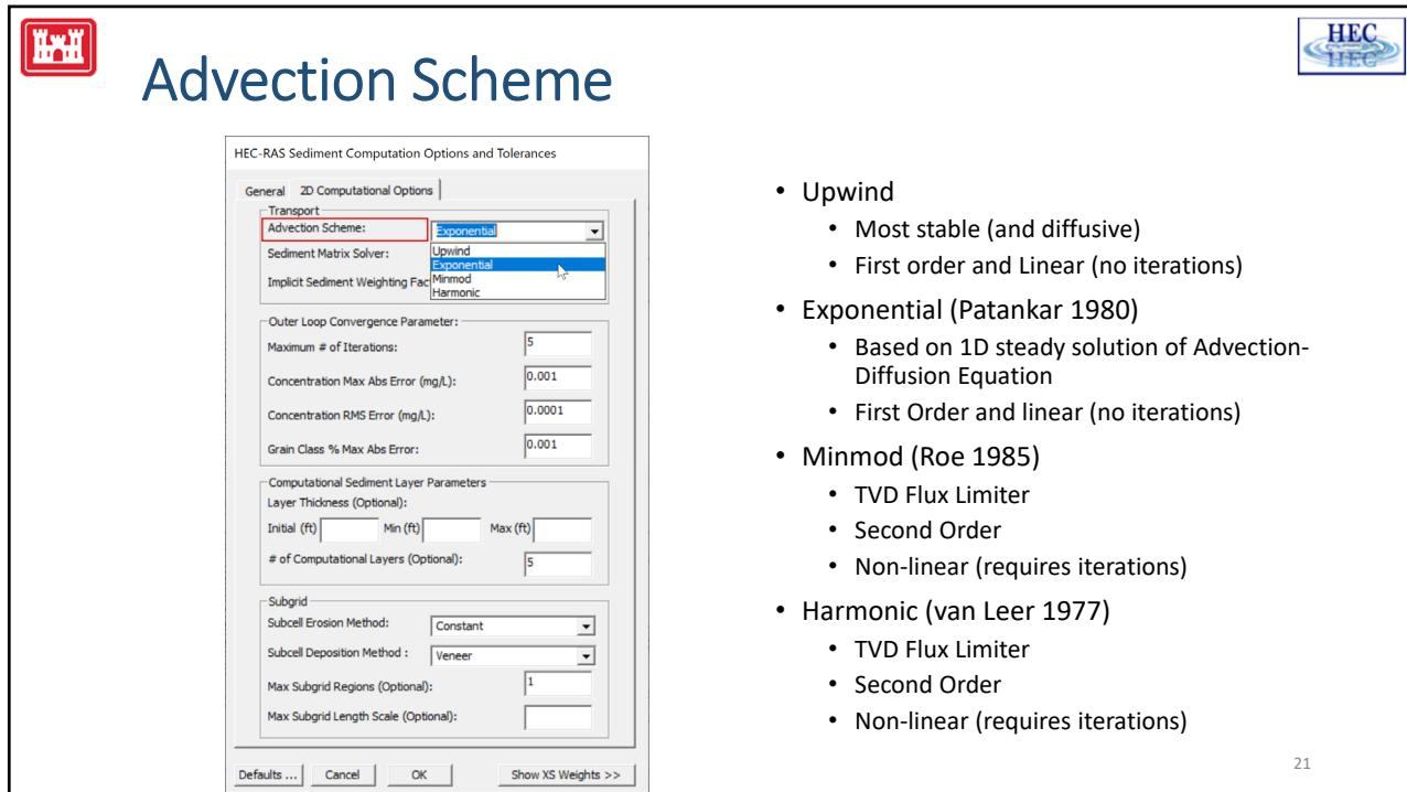
The screenshot shows the "Advection Scheme" dialog box from HEC-RAS. It displays various numerical methods for sediment transport. The "Advection Scheme" dropdown is set to "Exponential". Other options shown are "Upwind" and "Minmod". The dialog also includes settings for convergence parameters, sediment layer thickness, and subgrid erosion/deposition methods.
