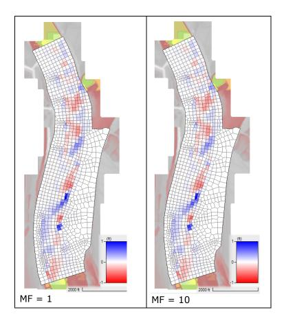
When comparing time-series of bed change of results which have the morphologic acceleration factor, it is necessary to scale time with the morphologic acceleration factor. This can be done by copy-pasting the data to excel and plotting it there. However, the finial values of the bed change can also be used to quickly identify differences in the results due to the MF.
