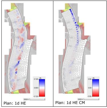
From the figure above it's clear that changing the computation multiplier caused the model to go unstable. This can be confirmed by looking at the **Computation Log File**. The figure below shows the convergence of the first two time steps.
