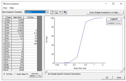
The sediment gradation has 5 grain classes. Two of these grain classes have 1% or less material (by weight). These grain classes can be ignored from the bed gradation.
