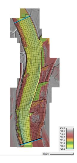
The base model has a constant flow upstream of 70,000 cfs, and a constant stage downstream of 172.936 ft. It is important to note, that though the current model setup may not be good for final production runs of a project, the sensitivity analysis as applied here with a fast model setup is useful and recommended for projects.
