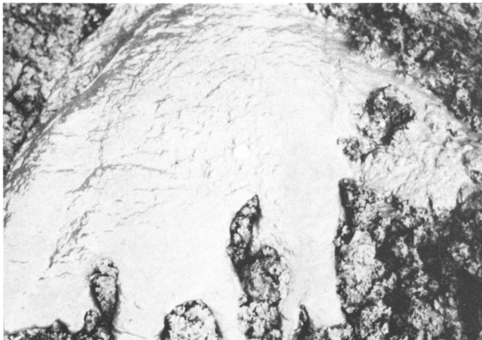
Fig.9. Soil and water flowing out of right descending bank, Ohio River, 662 km (411 miles) downstream from Pittsburgh, December 1977.
