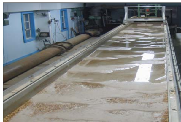
Drained flume following an experiment
