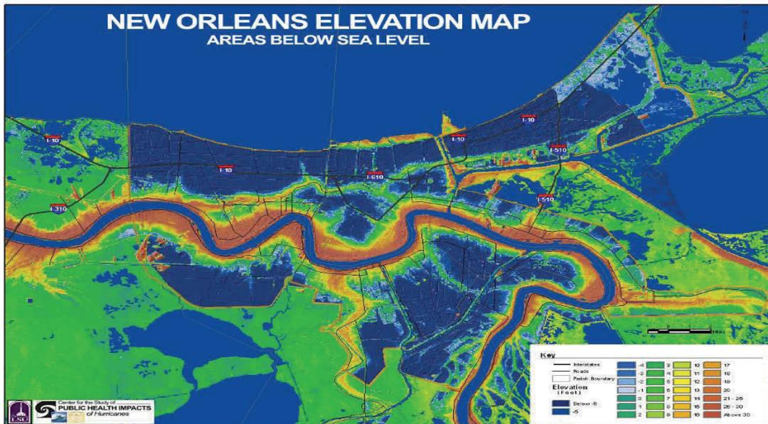
The modeling utilizes GIS-based data for definition of storage areas, location of external (ADCIRC) boundary conditions, comparison of computational results with observed high water marks, location of levee breaches and mapping of simulated flooded areas.
