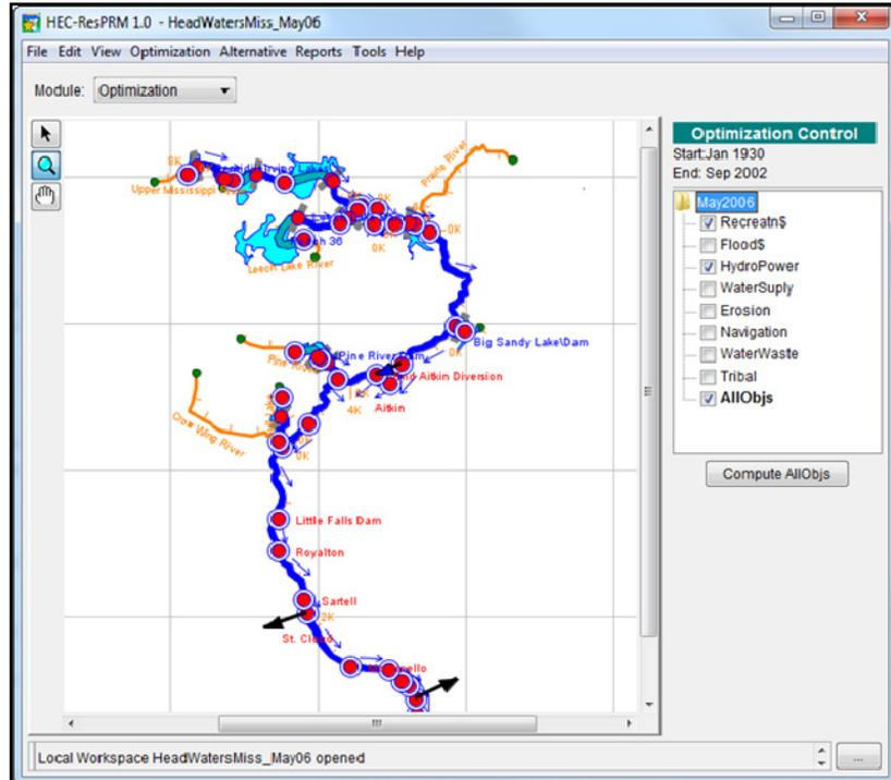
*This view of the HEC-ResPRM interface shows the optimization module with several different single-objective optimization scenarios, each focusing on a different interest. The individual objectives were also combined to form a multi-objective scenario that balances all interests.*
