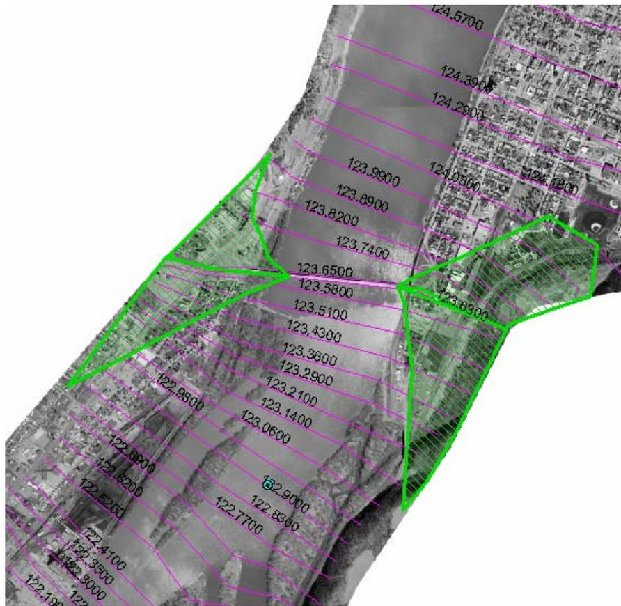
**Figure 4. Ineffective Area Polygon Layout in HEC-GeoRAS**
