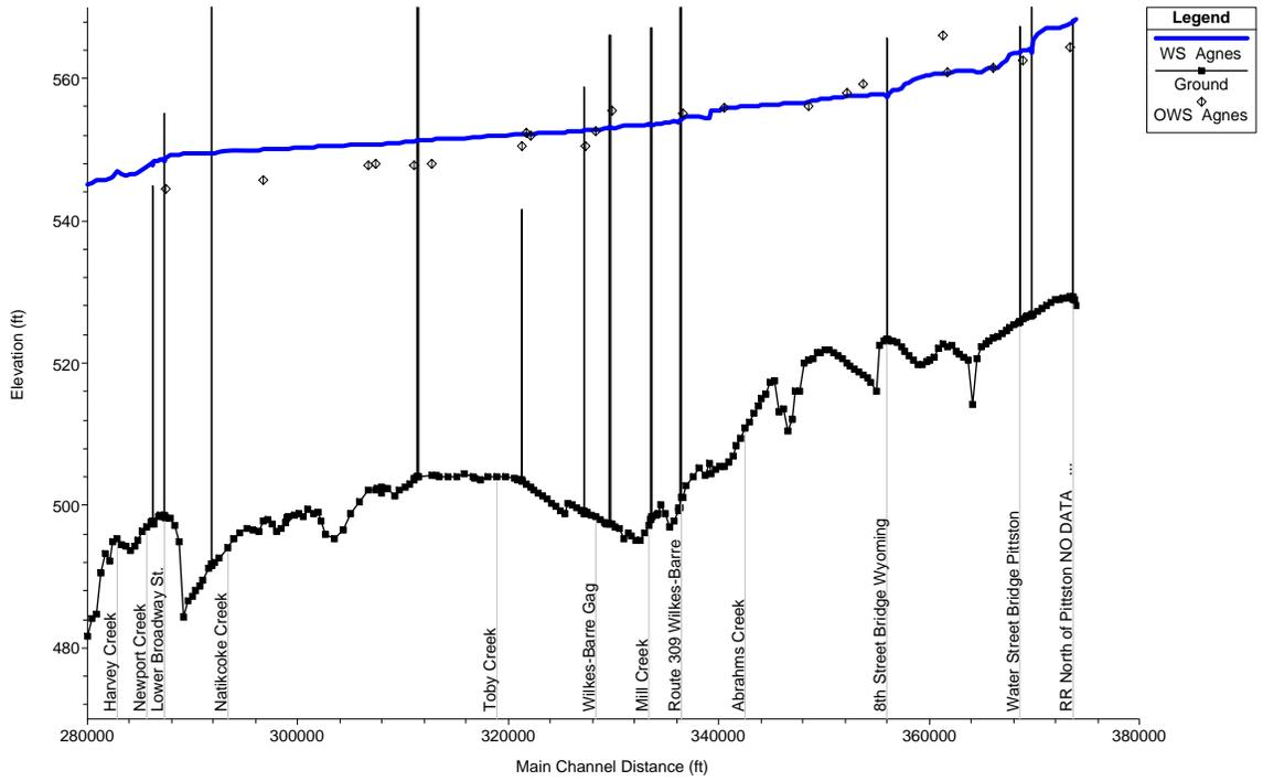
**Figure 5. Profile plot of the Agnes (1972) flood in Wilkes-Barre**
