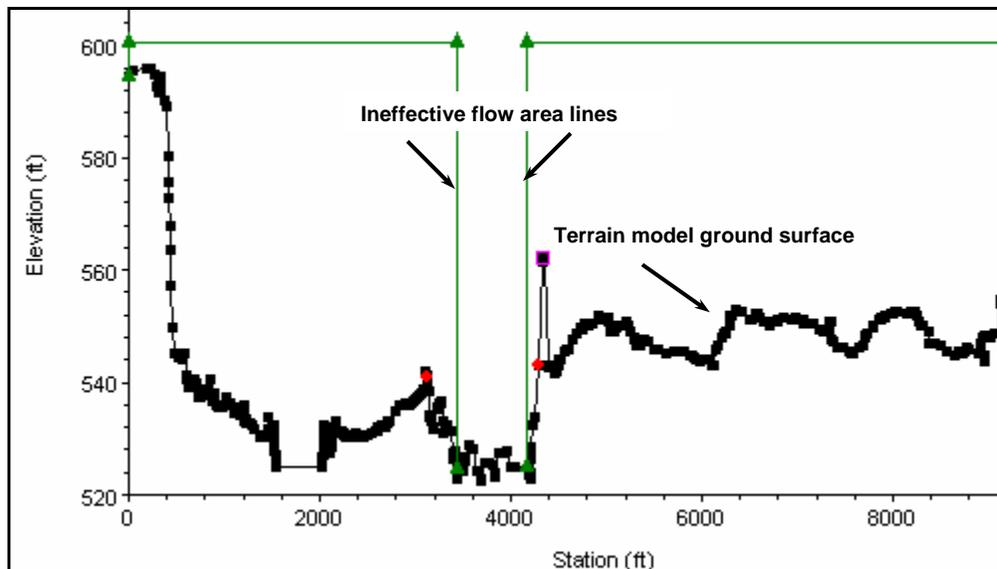
**Figure 1. Cross section with ineffective flow area lines indicating low flow channel. NOTE: The ineffective flow area lines were only used as markers between dry land and the channel surface at the time of the aerial survey.**
