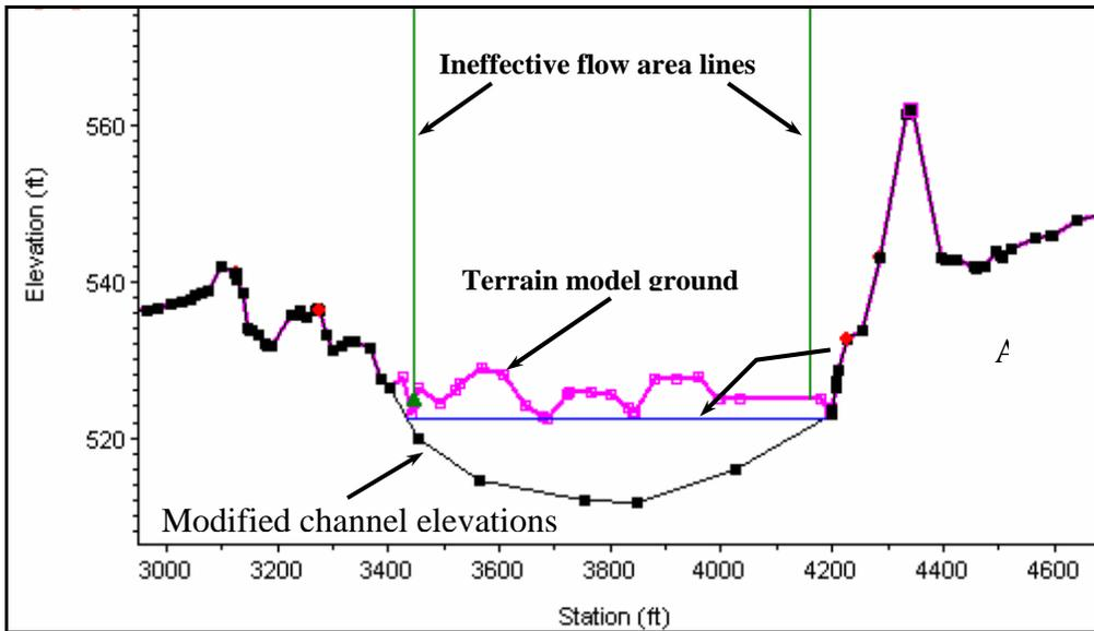
**Figure 2. Cross section with modified channel.**
