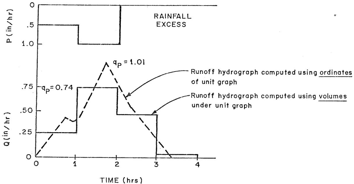
The difference in peaks between the ordinate derived and volume derived runoff hydrographs, 1.01 in/hr vs. 0.74 in/hr, demonstrates the reduction in peak discharge that can be expected from the way STORM applies the SCS triangular unit hydrograph.
