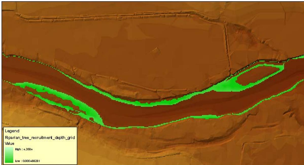
**Figure 49.** Depth grid created by clipping the inundation depth grid from the recruitment depth grid. The resulting area shows where HEC-EFM predicts Riparian tree establishment.
