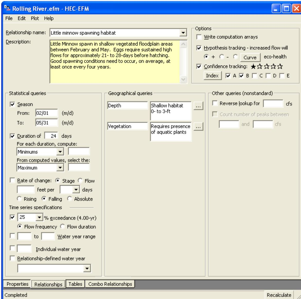
**Figure 3. Using the Relationships Tab of the main interface of HEC-EFM, modelers define individual relationships as combinations of statistical and geographical criteria.**
