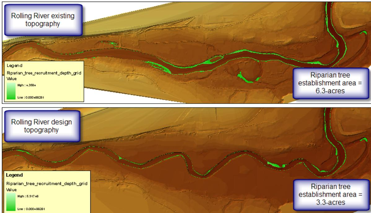
**Figure 52. Comparison of Riparian tree establishment in existing and restored topographic conditions.**
