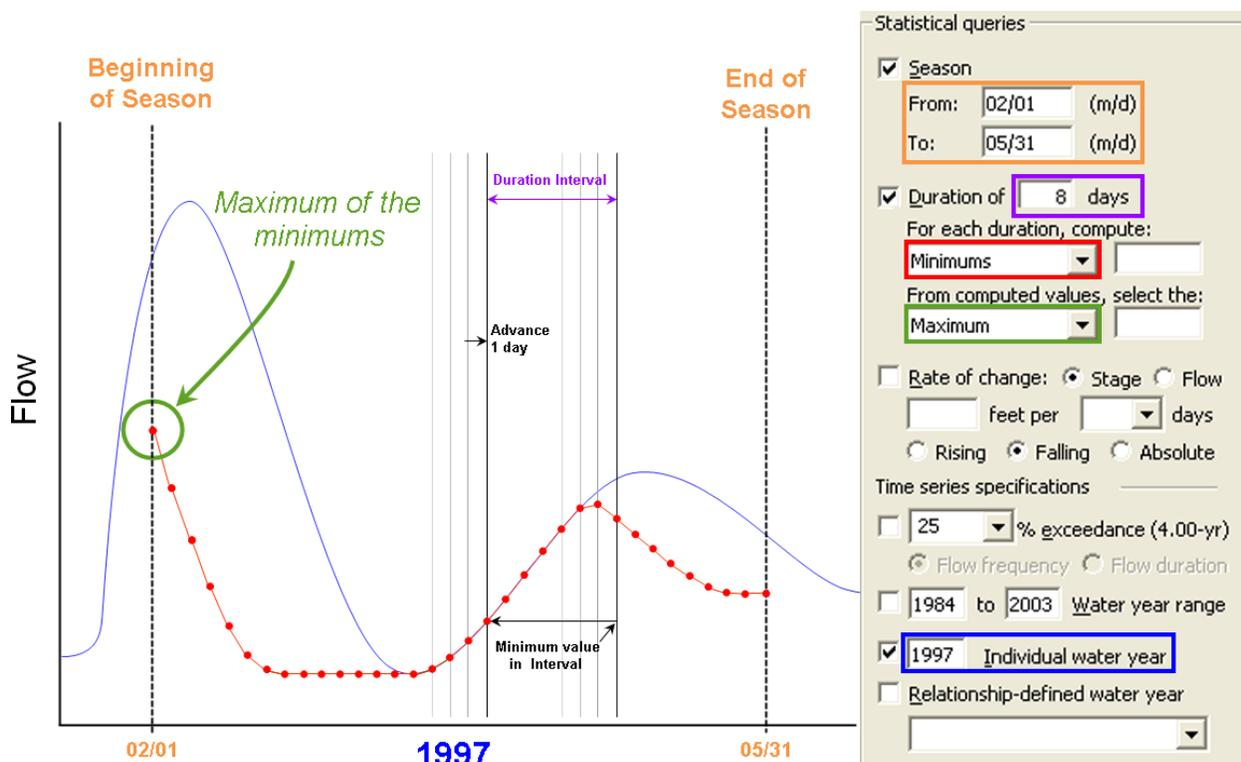
Figure 7. Sample use of the *Duration* query in HEC-EFM. Computations are shown for one water year.
