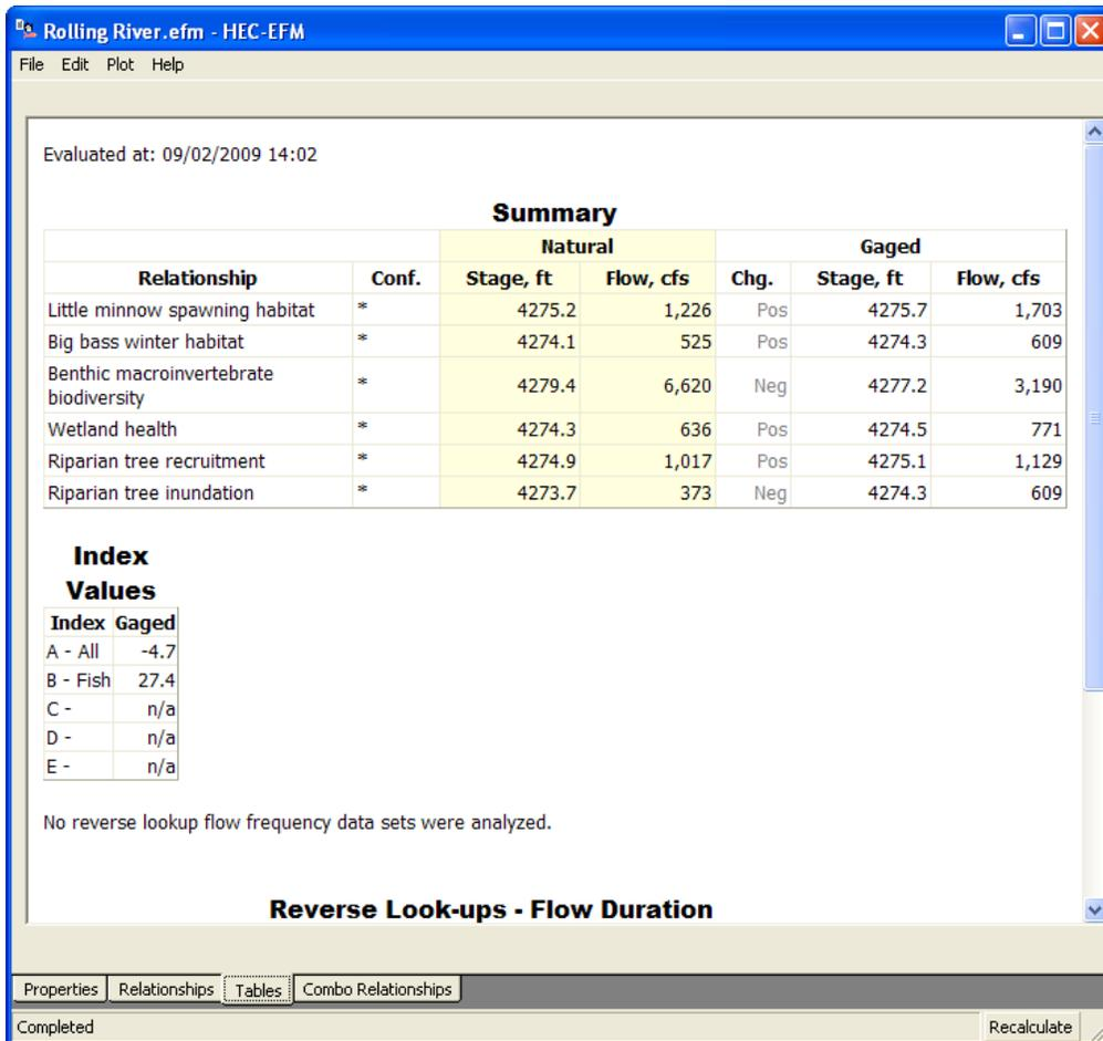
Figure 5. The *Tables Tab* of the HEC-EFM interface is used to display statistical results for simulations (as in this figure), project reports, and computational output.
