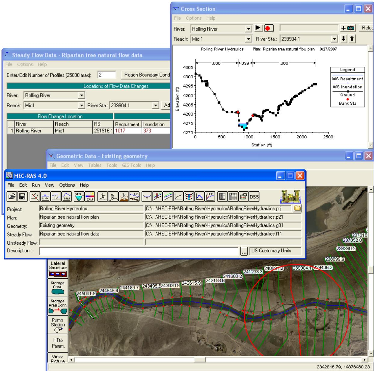
Figure 44. Example of HEC-RAS used to create water surface profiles for HEC-EFM statistical results (Riparian tree recruitment and inundation relationships using the Natural flow regime.)
