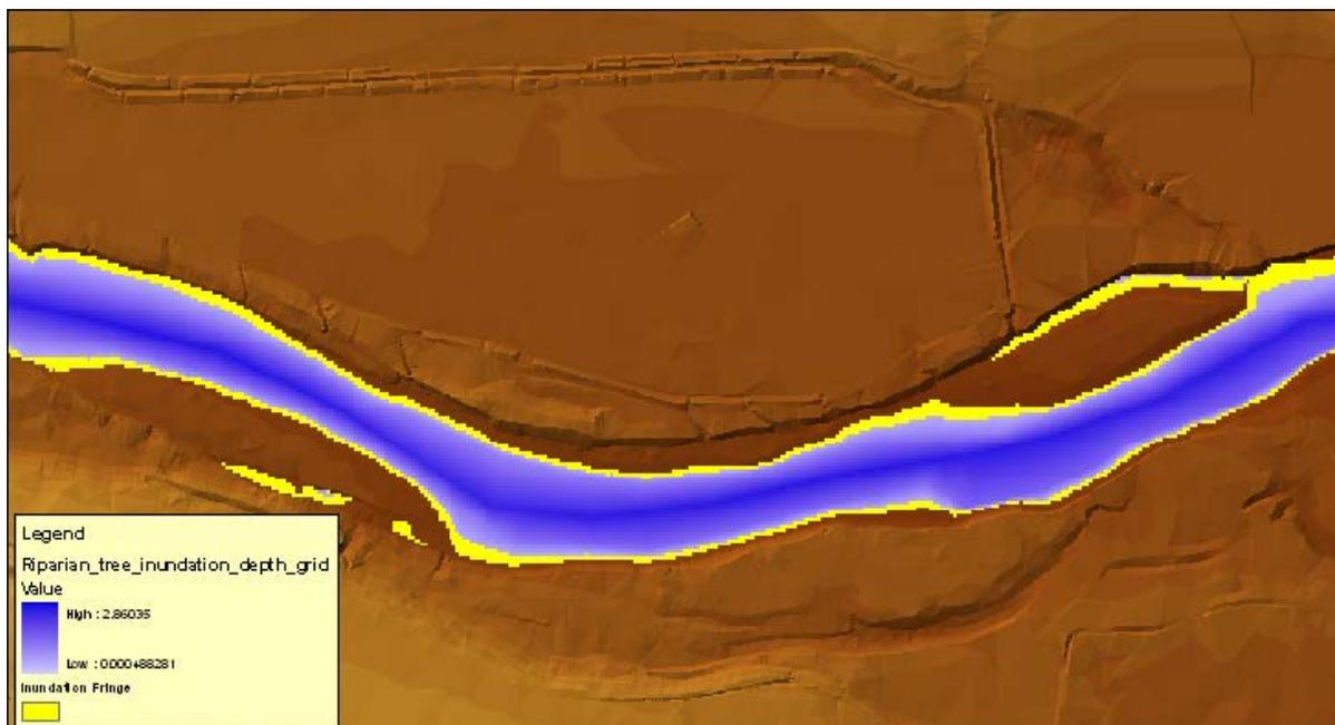
**Figure 50.** The yellow fringe shows areas of the Riparian tree inundation depth grid that are less than or equal to 0.5 ft, which may not be deep enough to drown new seedlings.
