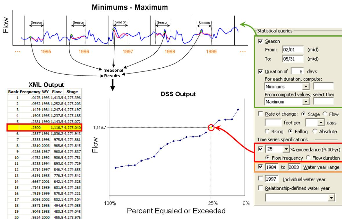
**Figure 9.** Sample use of the *Time series specifications* for a relationship with *Season* and *Duration* queries (as in Figure 7). The statistical result is the flow meeting the parameters in those queries that is equaled or exceeded in 25% of years (*Flow frequency*).
