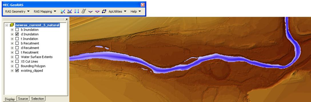
**Figure 45.** Example of a depth grid computed in HEC-GeoRAS using the water surface profile simulated by HEC-RAS for the statistical results of Riparian tree inundation from HEC-EFM.
