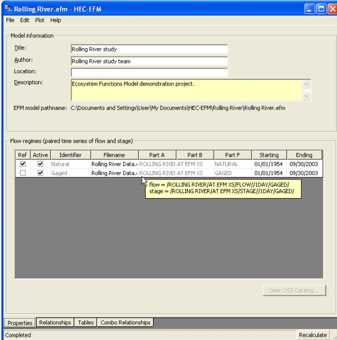
**Figure 2.** The *Properties Tab* of the main interface of HEC-EFM is used to document information about the project and to define the flow regimes to be analyzed. Two flow regimes (**Natural** and **Gaged**) are shown.
