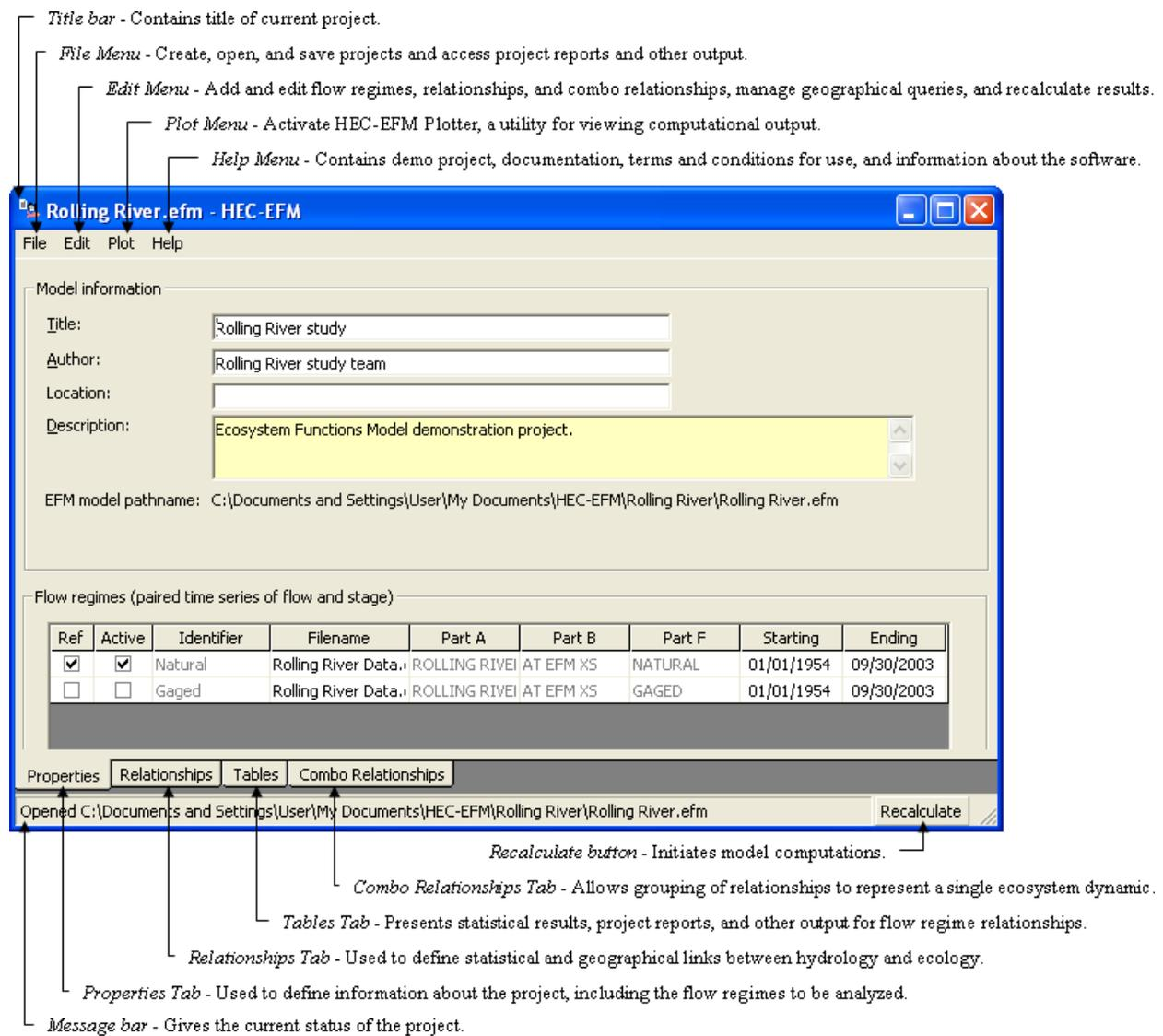
**Figure 1. Key components of the main interface of HEC-EFM.**
