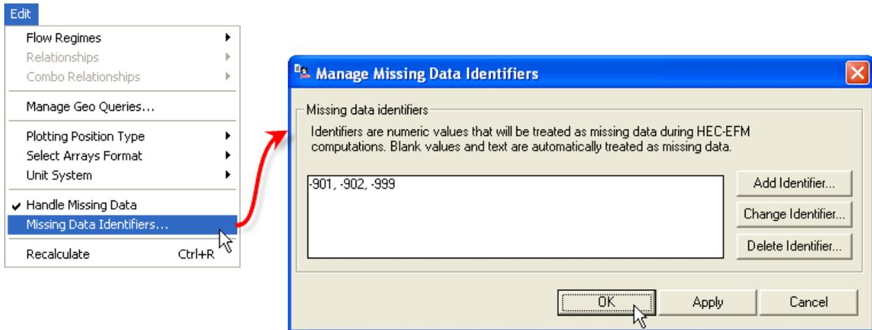
**Figure 14.** Use of the *Missing Data Identifiers* interface to specify the numeric values to be treated as missing data.
