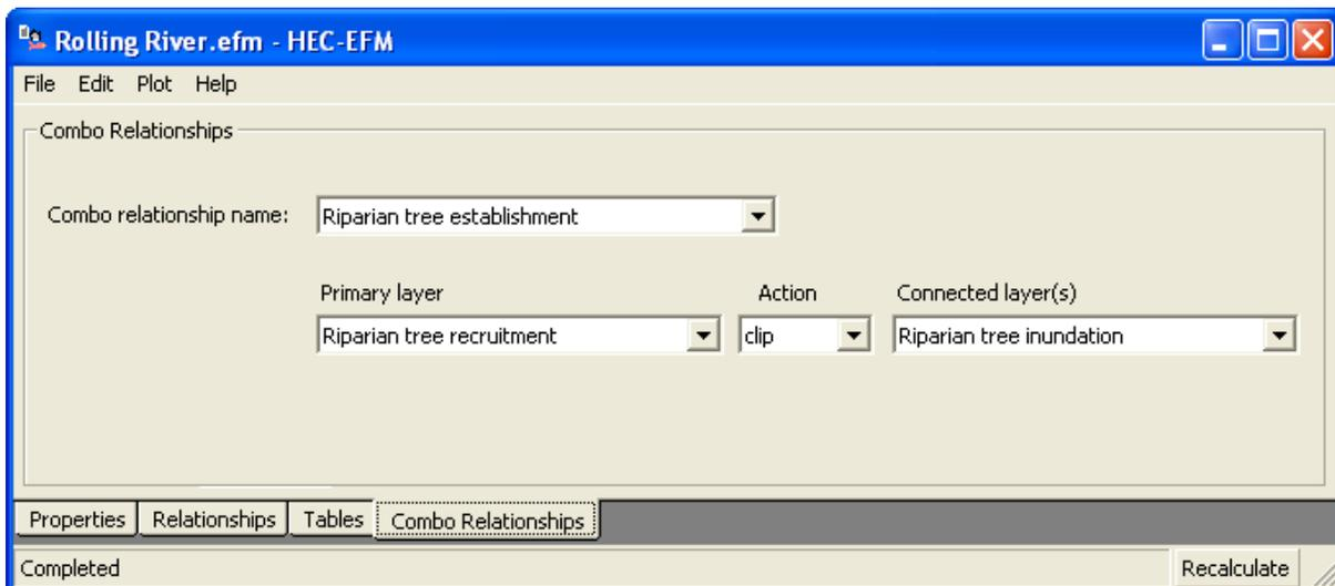
Figure 6. The *Combo Relationships Tab* of the HEC-EFM interface allows for grouping of separate relationships to represent a single ecosystem dynamic.
