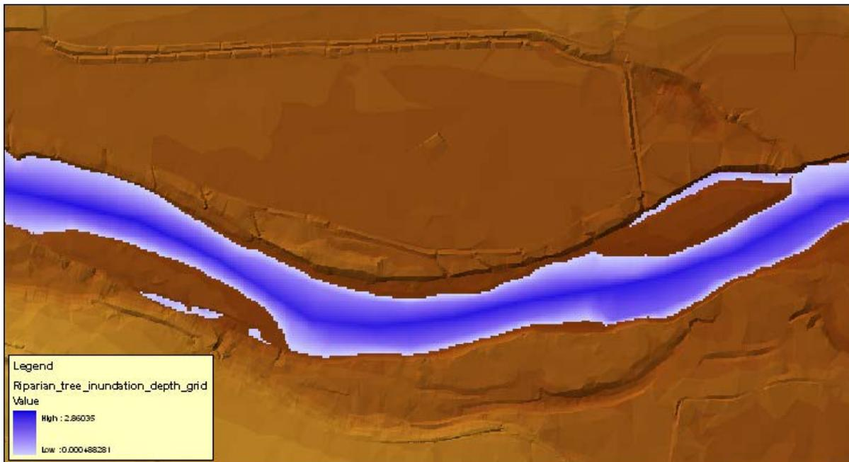
**Figure 47. Depth grid created for Riparian tree inundation. This blue area shows where any new seedlings will be drowned by prolonged inundation.**
