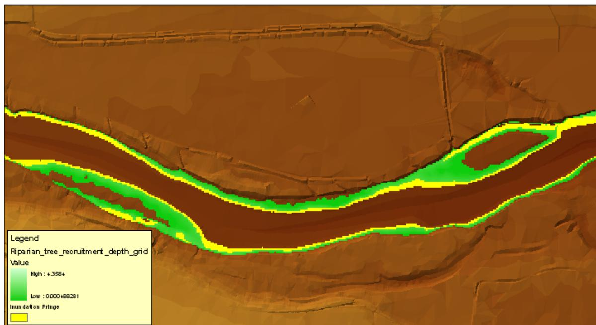
**Figure 51. Potential recruitment sites for the Rolling River's Natural flow regime as computed using statistical and geographical queries in HEC-EFM, water surface profiles computed by HEC-RAS, and depth grids produced by HEC-GeoRAS.**
