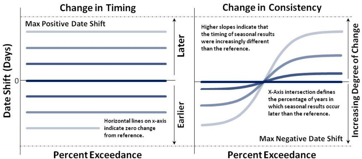
Figure 13. Date shifts provide insight regarding changes in the timing (left) and changes in the consistency of timing (right) of when criteria for a relationship were met. In HEC-EFM, “shifts” inherently compare an active flow regime with the reference flow regime. Date shifts are the time differences (numbers of days) between the seasonal date values of active and reference flow regimes.
