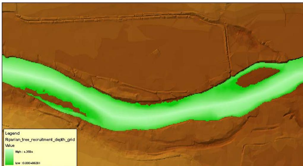
**Figure 46.** Depth grid created for Riparian tree recruitment. The green area shows where stage recession creates suitable conditions for seedlings to begin to grow.
