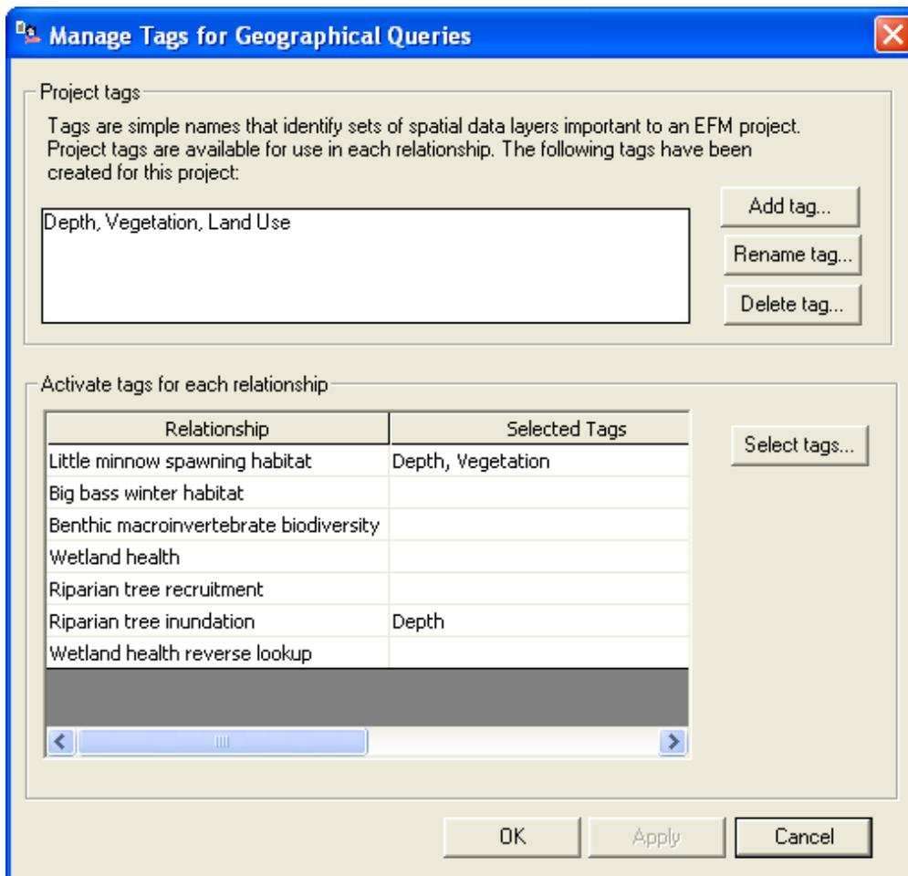
**Figure 4.** The *Manage Tags for Geographical Queries* interface in HEC-EFM is used for editing and creating tags, which are labels for sets of spatial data important to an HEC-EFM project.
