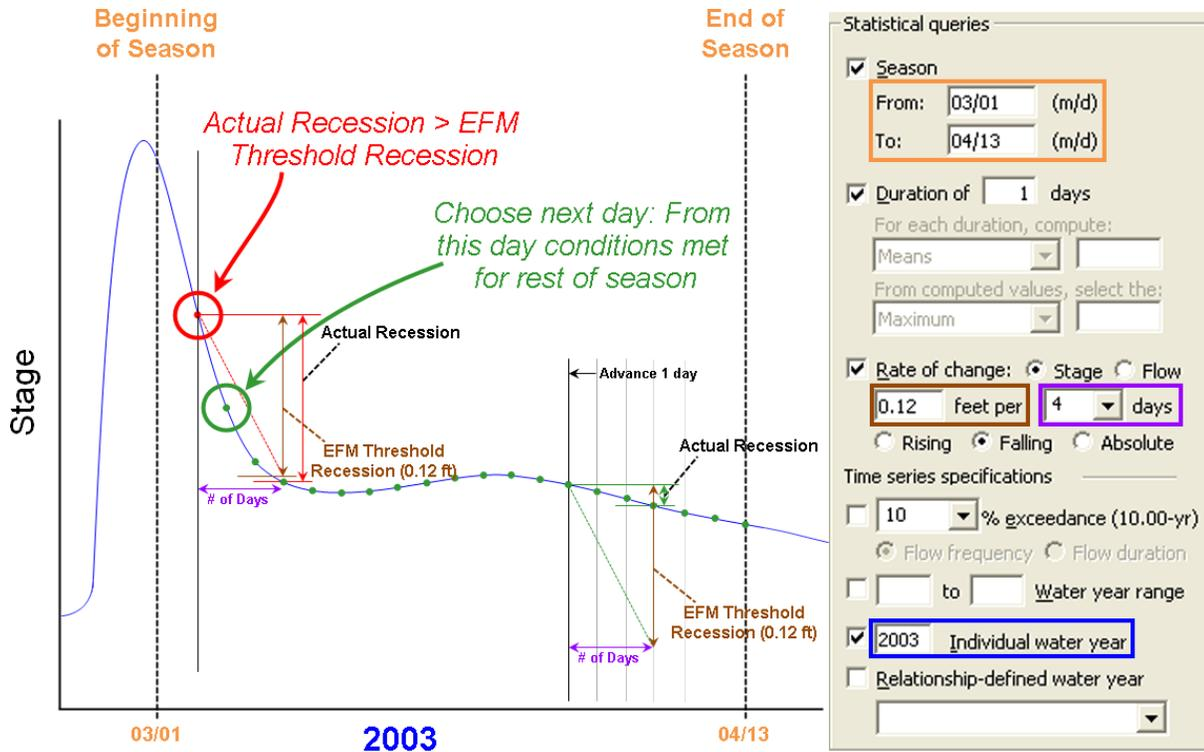
**Figure 8. Sample use of the *Rate of change* query in HEC-EFM. Computations are shown for one water year.**
