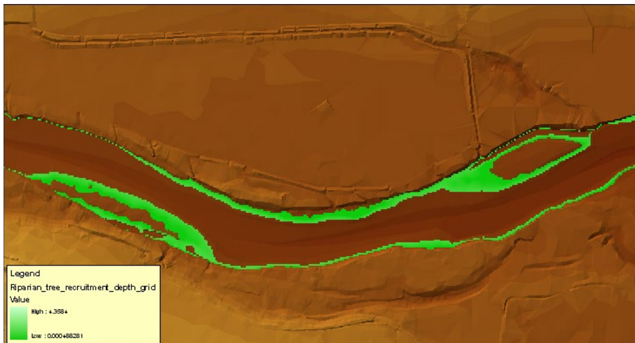
Figure 55. Depth grid created by clipping the inundation depth grid from the recruitment depth grid. The resulting area shows where HEC-EFM predicts Riparian tree establishment .
