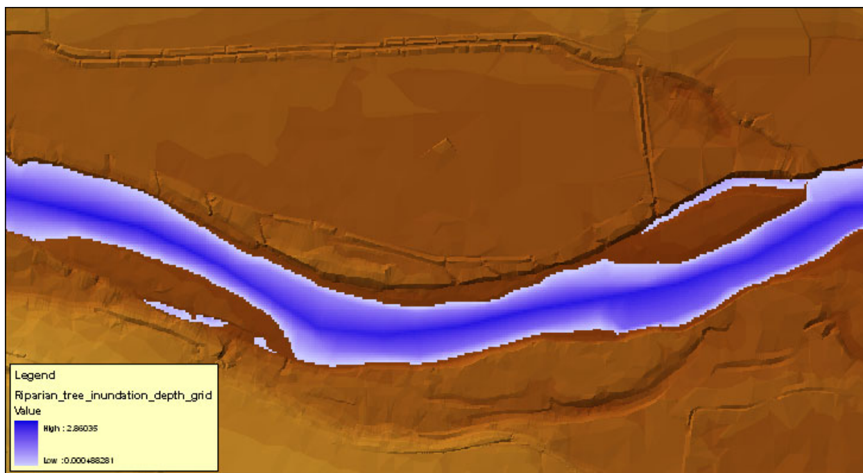
Figure 53. Depth grid created for Riparian tree inundation . This blue area shows where any new seedlings will be drowned by prolonged inundation.
