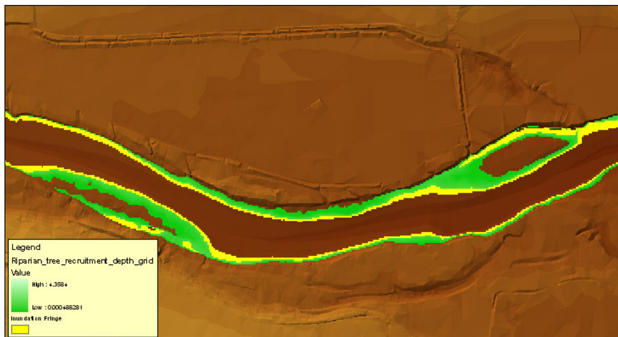
Figure 57. Potential recruitment sites for the Rolling River's Natural flow regime as computed using statistical and geographical queries in HEC-EFM, water surface profiles computed by HEC-RAS, and depth grids produced by HEC-GeoRAS.
