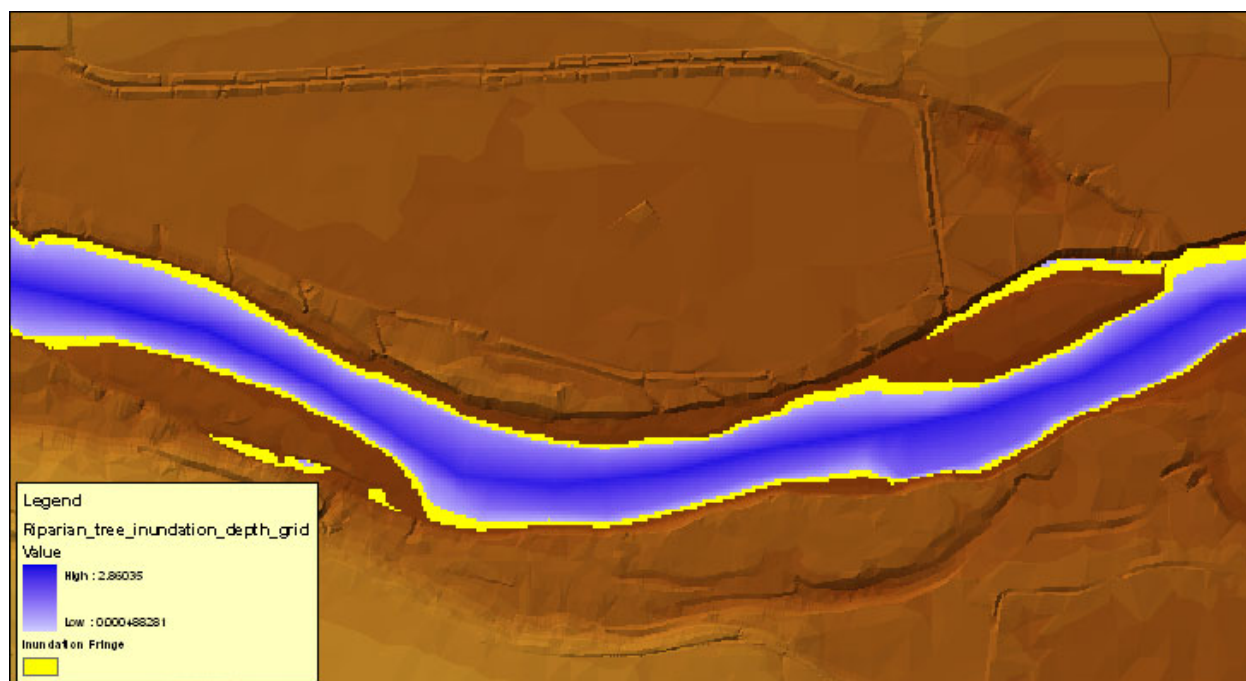
Figure 56. The yellow fringe shows areas of the Riparian tree inundation depth grid that are less than or equal to 0.5 ft, which may not be deep enough to drown new seedlings.
