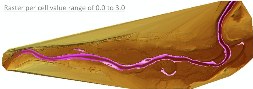
*Figure 5. Top image shows a depth raster (blue) from a river hydraulics model. Bottom image show raster of depths from 0.0 to 3.0.*
