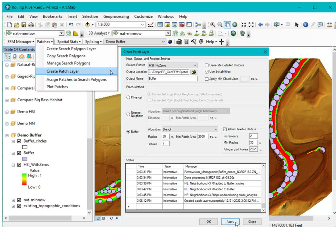
Figure 9. Creating a patch layer using the GeoEFM buffer method.
