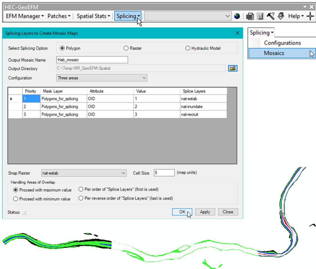
Figure 12. The splicing interface allows users to select and apply combinations of configuration, snap raster, and overlap option to create raster mosaics.
