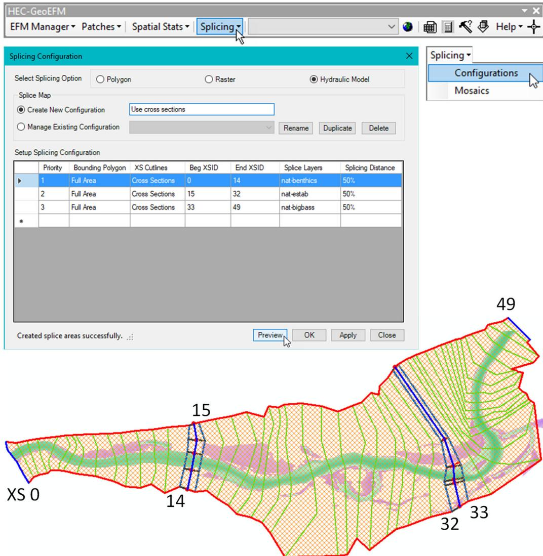
Figure 11. Interface for and preview of a hydraulic model splicing configuration.
