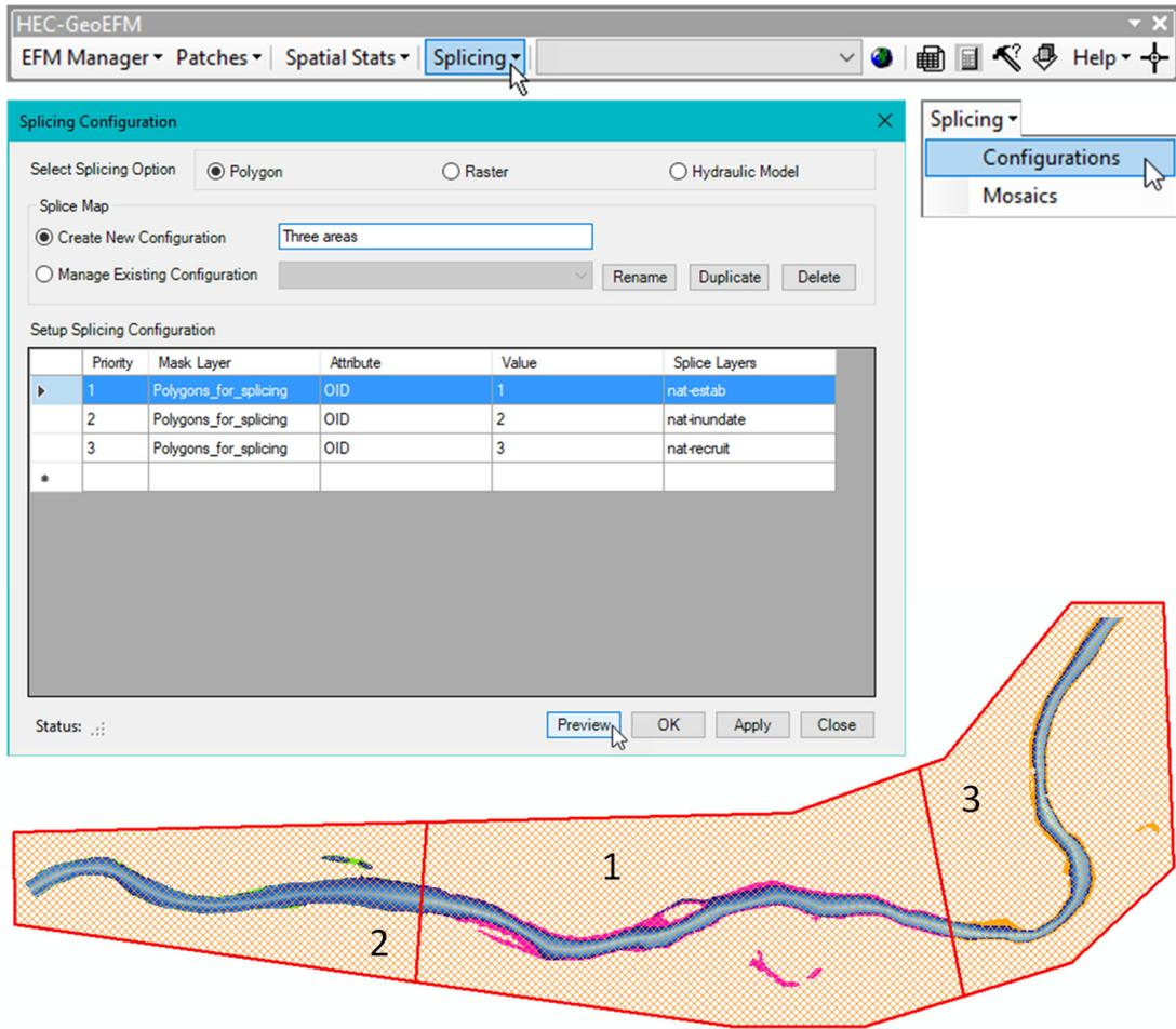
Figure 10. Interface for and preview of a polygon splicing configuration.
