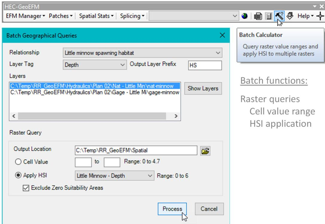
Figure 6. GeoEFM Batch Calculator interface being used to apply a HSI to multiple raster layers.
