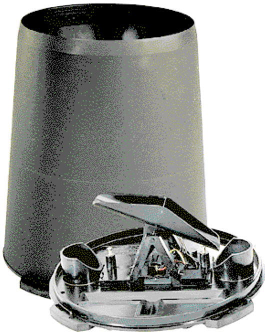
1 Figure 10. Telemetering precipitation observation gage
