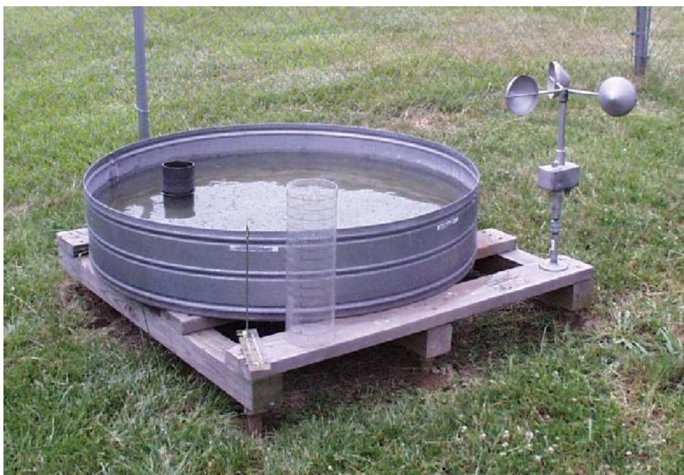
Figure 24. Example installation of a Class A evaporation pan.
