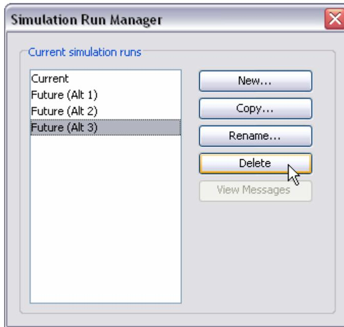
Figure 182. Preparing to delete a simulation run from the Simulation Run Manager. A confirmation will be required after pressing the **Delete** button.
