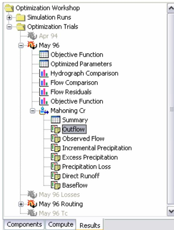
Figure 214. Viewing optimization results in the Watershed Explorer. The summary table is available for each element above the optimization location. Actual time-series are also available for each element.
