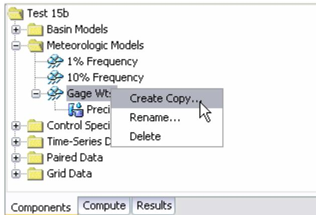
Figure 142. Copying a meteorologic model from the *Watershed Explorer*. The *Copy Meteorologic Model* window will appear after the **Create Copy...** menu command is selected.
