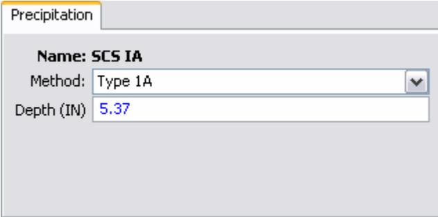
Figure 163. Precipitation component editor for the SCS storm precipitation method.
