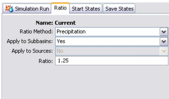
Figure 185. Entering a precipitation ratio for all of the subbasins in the simulation run. If a flow ratio were selected, it could be applied to subbasins or sources or both subbasins and sources.
