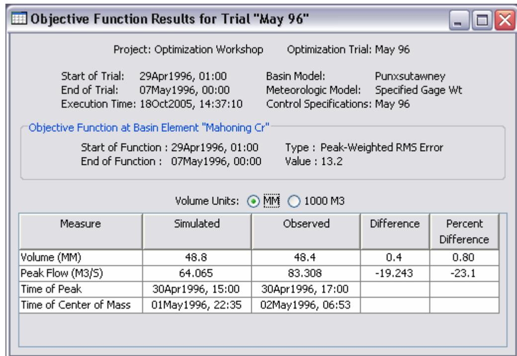
Figure 208. Objective function table for an optimization trial. The table presents statistical results of the computed and observed flow at the optimization location.
