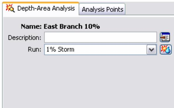
Figure 224. Depth-area analysis component editor where the simulation run used for the analysis can be selected.
