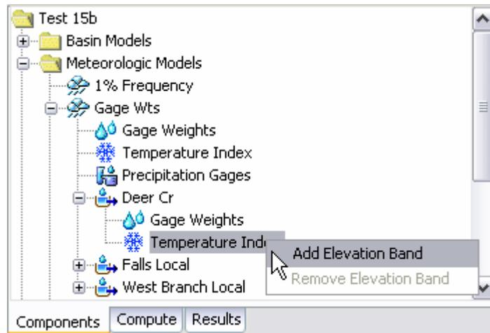
Figure 174. Adding an elevation band to a subbasin.
