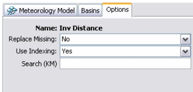
Figure 159. Selecting options for the inverse distance precipitation method.
