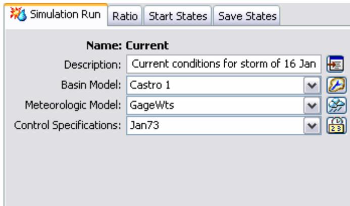
Figure 184. The simulation run component editor can be used to change a selected component after the run has been created.
