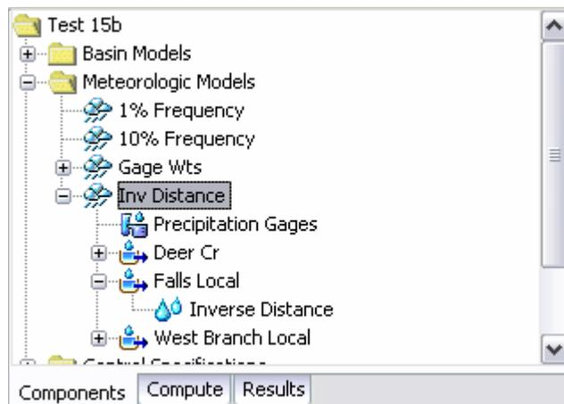
Figure 160. View of a meteorologic model in the Watershed Explorer when the inverse distance precipitation method is selected. Options are selected as shown in Figure 159.
