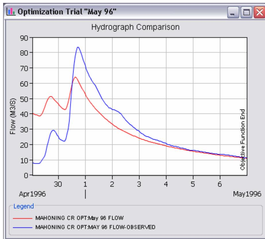
Figure 210. Hydrograph comparison graph showing the computed and observed flow at the optimization location.
