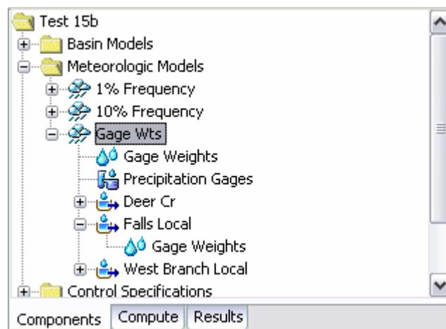
Figure 152. View of a meteorologic model in the Watershed Explorer when the gage weights precipitation method is selected. Options are selected as shown in Figure 151.
