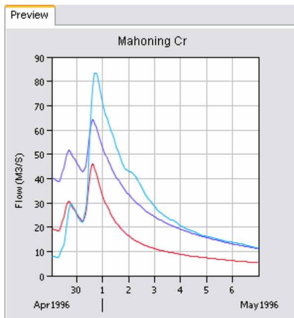
Figure 215. Preview graph showing computed outflow and observed flow from one optimization trial plus computed outflow from a different trial.
