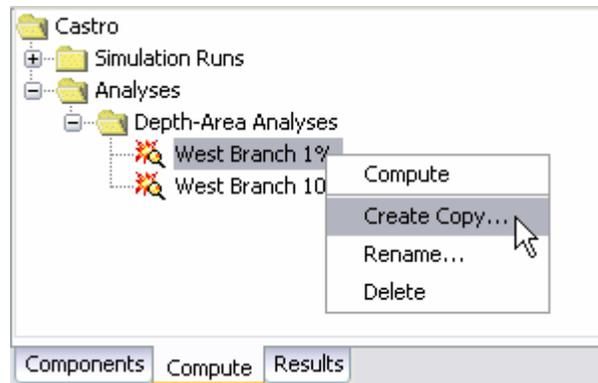
Figure 219. Copying an analysis from the Watershed Explorer. The Copy Analysis window will appear after the **Create Copy...** menu command is selected.
