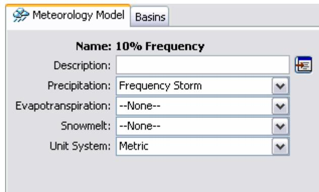
Figure 147. Meteorologic model component editor for selecting the precipitation, evapotranspiration, and snowmelt methods.
