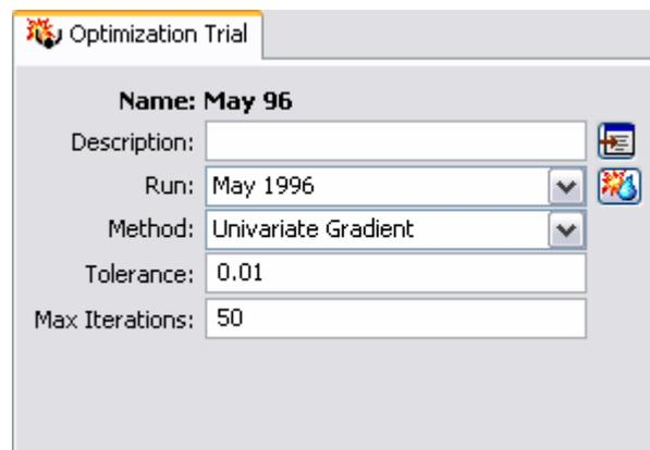
Figure 203. The optimization trial component editor can be used to change the run used in a trial, to select the search method, and to control the search tolerance.
