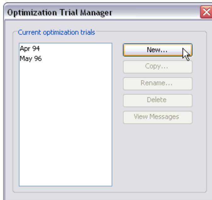
Figure 195. Beginning the process of creating a new optimization trial using the *Optimization Trial Manager*.
