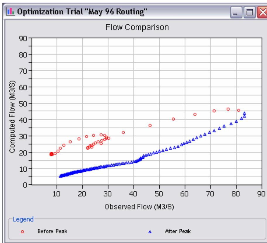
Figure 211. Flow comparison graph showing the computed flow plotted against the observed flow. Different symbols are used for points before and after the observed peak flow.
