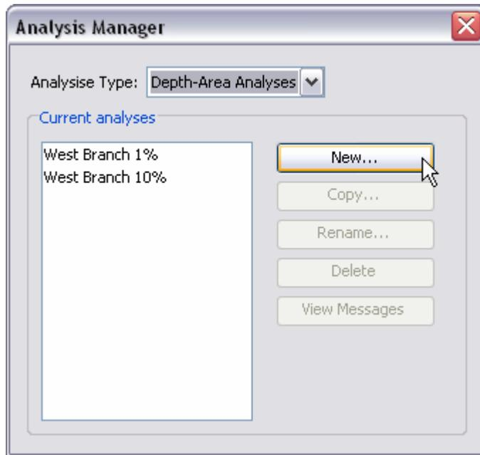
Figure 216. Beginning the process of creating a new depth-area analysis using the Analysis Manager. Create a different type of analysis by first selecting the desired type.
