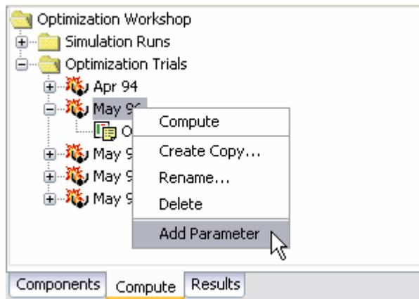
Figure 205. Adding a parameter to an optimization trial.
