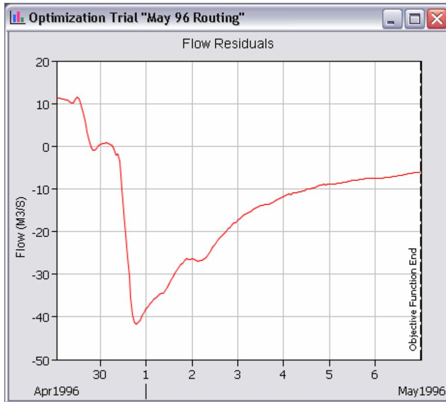
Figure 212. Flow residuals showing the computed minus the observed flow at the optimization location.
