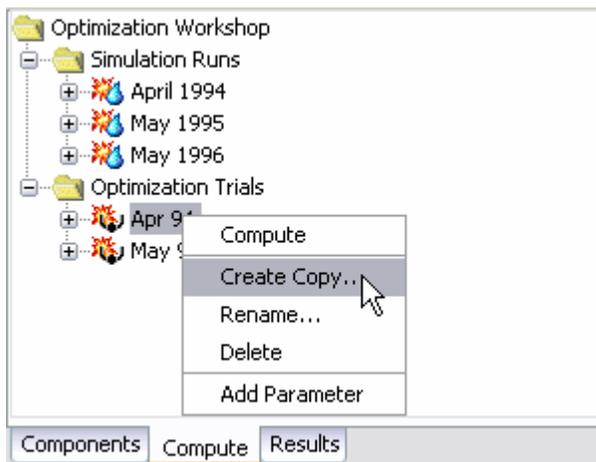
Figure 198. Copying an optimization trial from the *Watershed Explorer*. The *Copy Optimization Trial* window will appear after the **Create Copy...** menu command is selected.
