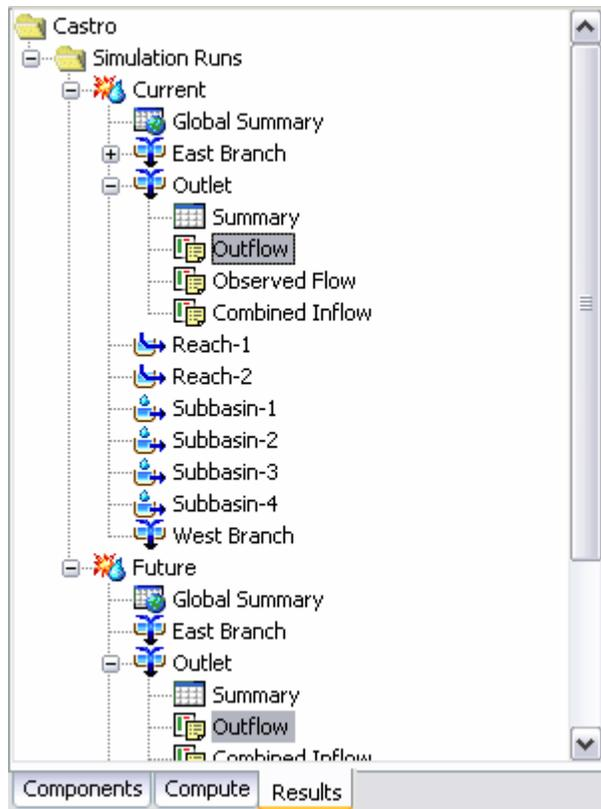
Figure 193. Selecting computed outflow from the same element in two different simulation runs. Other types of time-series data could also be selected.
