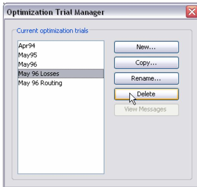
Figure 201. Preparing to delete an optimization trial from the *Optimization Trial Manager*. A confirmation will be required after pressing the **Delete** button.
