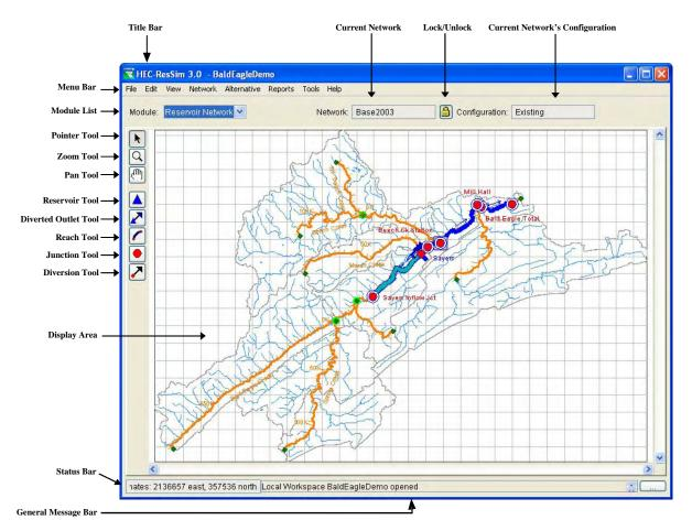
Figure 8.1 Reservoir Network Module Main Window
