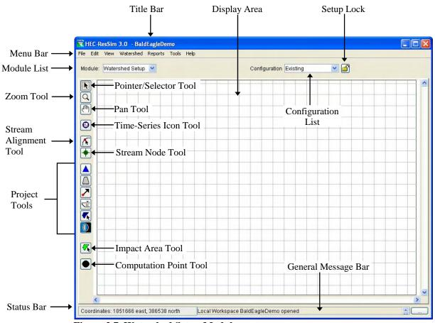
Figure 2.7 Watershed Setup Module
