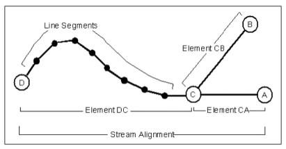
Figure 5.5 Relationship of Line Segments, Stream Elements, and Stream Alignment
