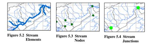
When you create a Stream Alignment, you draw it as a set of connected, multi-segmented lines. The Stream Alignment must have at least two nodes, defining the beginning and end of a stream element. Figure 5.5 illustrates the relationship of line segments, stream elements, and the Stream Alignment.
