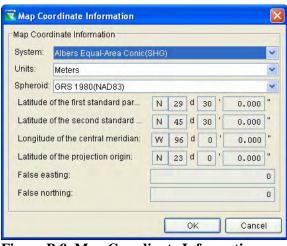
Figure B.9 Map Coordinate Information, Albers Equal-Area Conic (SHG) System
