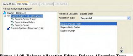
Figure 11.98 Release Allocation Editor, Release Allocation Type for *Dam* is *Sequential* for Three Outlets
