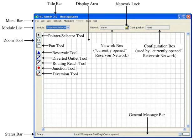
Figure 2.8 Reservoir Network Module
