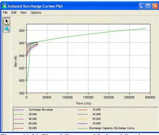
Figure 11.24 Plot of Computed Induced Surcharge Curves (*with* the Discharge Capacity Discharge Curve)
