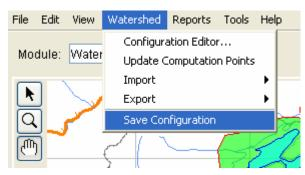
Figure 8.22 Watershed Setup Module - Watershed Menu: Save Configuration before Updating Network
