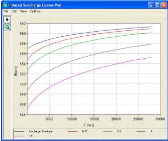
Figure 11.27 Plot of Computed Induced Surcharge Curves (without the Discharge Capacity Discharge Curve)
