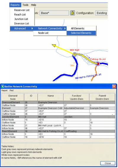
Figure 8.20 Reservoir Network Reports: Advanced --Network Connectivity – "Selected" Elements"
