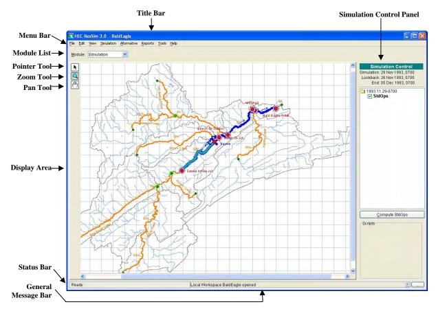
Figure 14.1 Simulation Module Main Window
