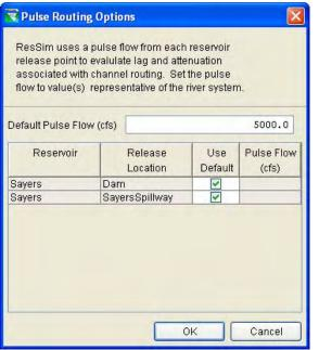
Figure 10.51 Dam Component: Pulse Routing Options Editor
