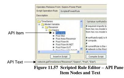
4. Developing the script involves writing Jython code to create the data objects and execute the methods and other calculations that will produce a desired release limit to be returned by your rule. It is important to note that a scripted rule is essentially a Release Function rule; thus, the rule must return a desired "release" value and an associated "Limit Type" for that release value. The limit types are Maximum, Minimum, and Specified.
