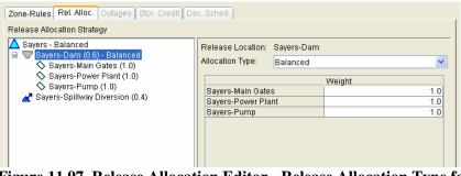
Figure 11.97 Release Allocation Editor - Release Allocation Type for Dam is Evenly Balanced between Three Outlets
