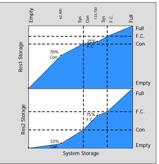
Figure 12.6 Explicit System Storage Balance
