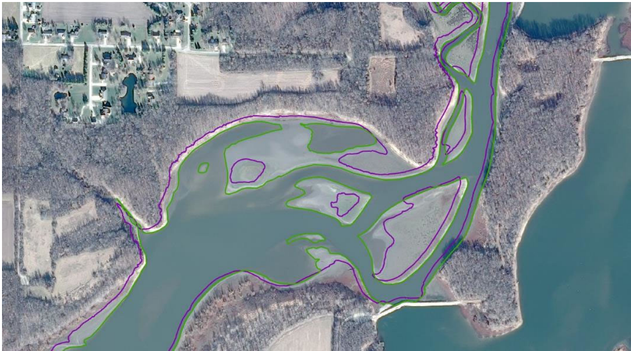
Figure 17. Drawdown aerial imagery for a section of Lake Shelbyville bankline with guide curve (purple) and 0.5 ft drawdown (green) waterlines delineated.
