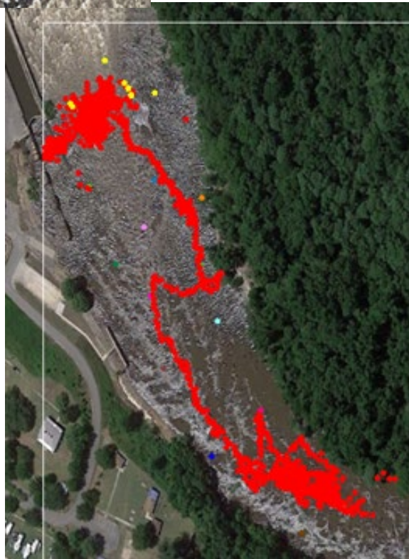
Figure 10. Striped bass telemetry from May 30, 2021, monitoring by Clemson University. Fish navigated rock ramp in 48 minutes.
